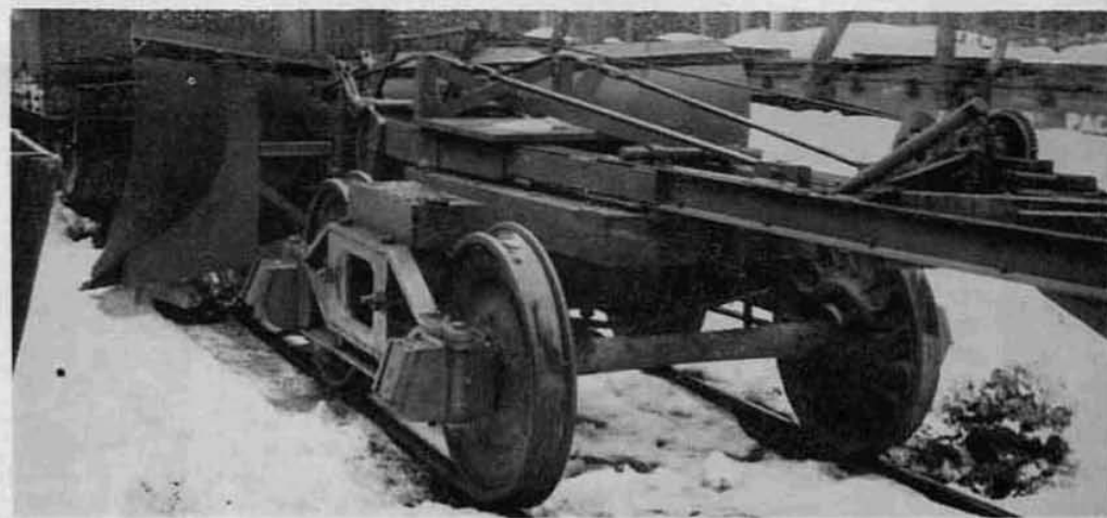
Below—Close-up of plow. It is light enough that any one of the camp speeders can push it.
