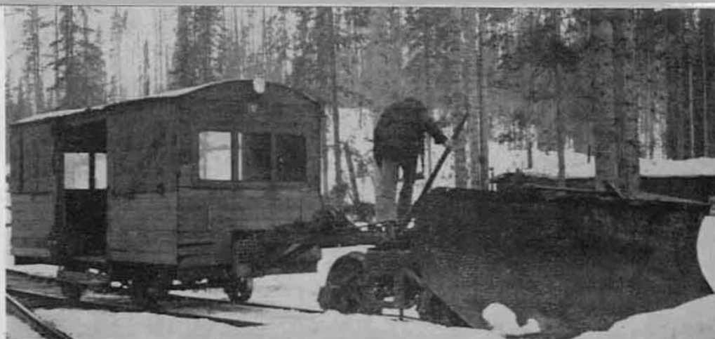
A new snowplow, which works very efficiently in light snow up to a depth of nine or ten inches, has been developed at Headquarters. The inventors are Charlie Horne, trainmaster, and Henry Hemly, master mechanic for the truck shop. The plow is mounted on the trucks taken from an old freight car and is so balanced from a center pivot spot that it can be reversed at will.
