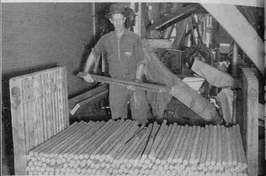
Left—Sticks of compressed waste cedar, five at a time, are extruded from the Pres-to-logs stoker machine. Above—Ward Tousley, engineering department, supervises operation of the machine, breaks the sticks into handy four-foot lengths for loading.
