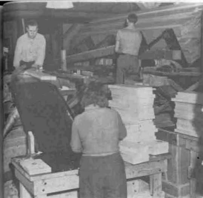
Above—Lumber is cut to proper length for shook by push cut-saws. Saw operators work on a platform above the floor level. Lumber is hoisted to them in unit lots by push button controlled hoists which can be tilted to keep boards always within easy reach. They drop from saw down a metal chute to off-bearer.
