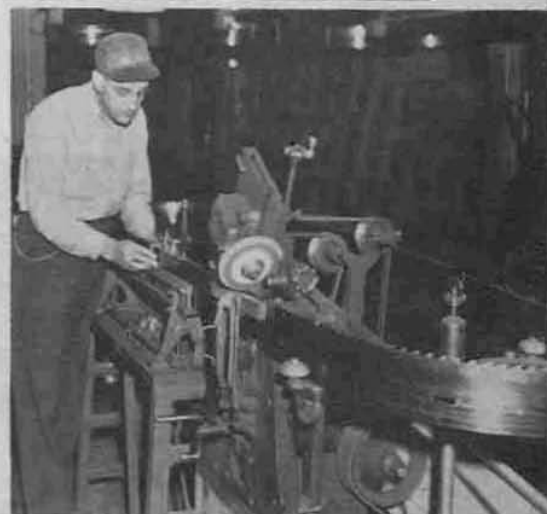
Above—Twin, upright resaws, manufactured by the Turner Mfg. Co., San Francisco, have been installed in the Clearwater Box Factory. Four cuts of a single board are possible (making five pieces) and a splitter attachment that serves as a rip saw makes possible further division of the board into desired width slats. The machines are set to saw in tandem or individually. Automatic feeds have been ordered but have not as yet arrived.
