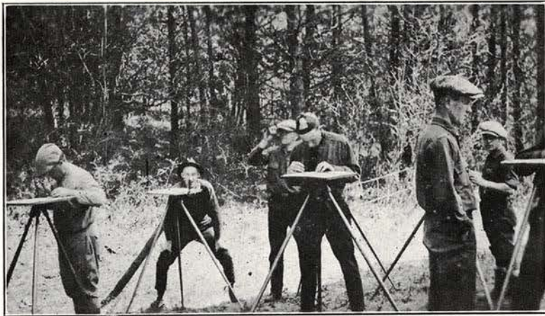
Class in Forest Surveying with Traverse Boards
