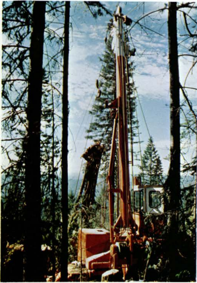
Madill Model 078 West Coast Tower working in a configuration of a side mount tower.
