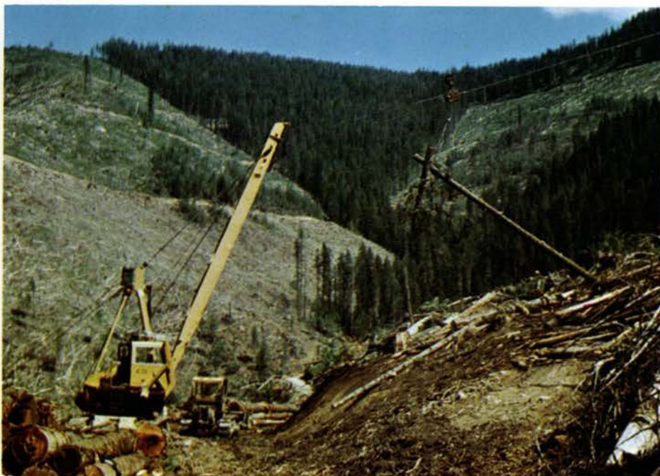
Running skyline Skylock Model 78 working on burn near Elk River.
