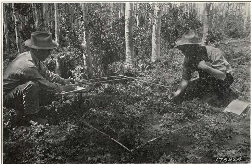
Fig. 4. Mapping a Quadrat with the Hill Chartograph. This device which adapts the use of the ordinary Pantograph to quadrat work, greatly speeds up, adds to the accuracy and removes much of the tedium in quadrat mapping.
