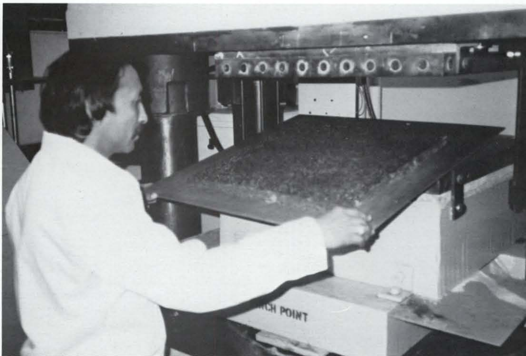
A wood-cement composite being made in the Department of Forest Products laboratory in its computerized press. It is then examined for surface quality and other properties. A.A. Moslemi
