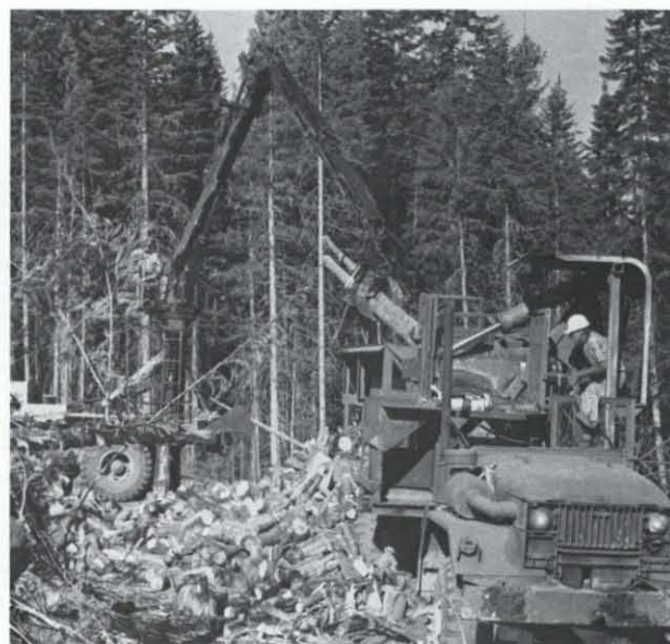
Firewood in 18-inch lengths was produced by this hydraulic shear from the wood waste left after timber cutting. Leonard Johnson
