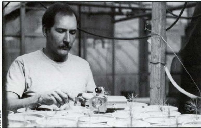
How much water are these eight-week-old ponderosa pines losing in the process of photosynthesis? Peter Kolb uses a LiCor porometer to measure the seedlings' changes in humidity.
