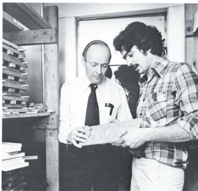
John Howe, left, and Manoel Sobral examine board samples made from a combination of round wood and pulp chip strands. Dave Hoffman photo
