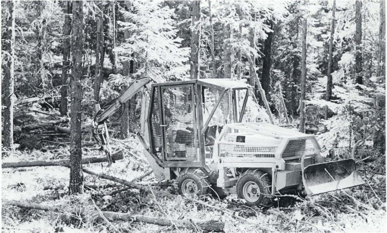
A small-wheeled skidder has been developed from a Case-Davis 30-horsepower backhoe. The machine's backhoe has been modified for grappling logs. Leonard Johnson photo
