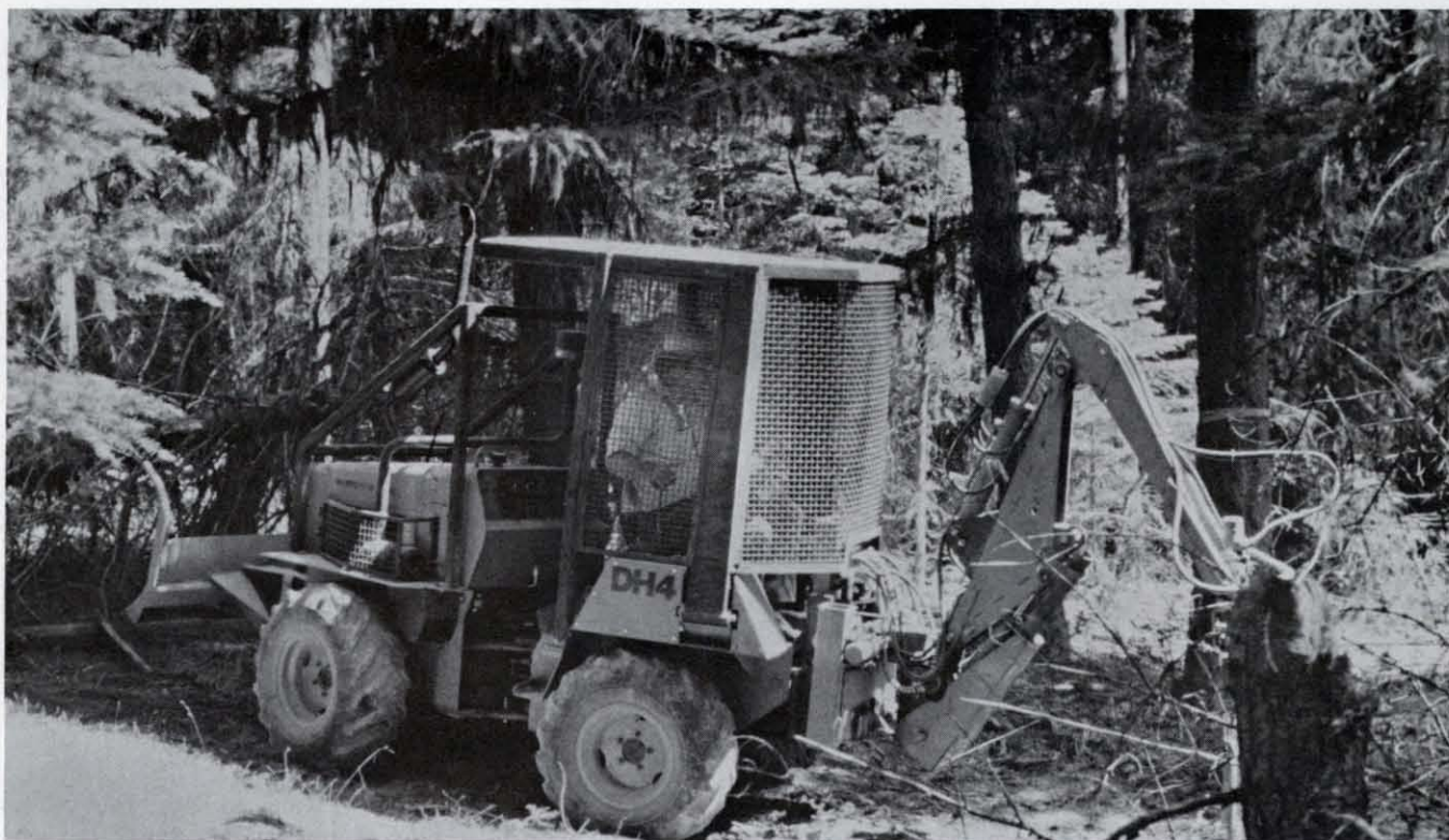
Scientists in Forest Products and Agricultural Engineering are using this 40-horsepower Case diesel backhoe to remove small diameter trees from precommercial thinnings on the University of Idaho Experimental Forest. The modified skidder will be tested through the fall logging season. Leonard Johnson photo
