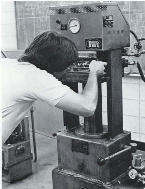
Dave Ritter checks the alignment of wood flakes and frame before pressing a sample board in the Forest Products laboratory. Susan Roberts photo
