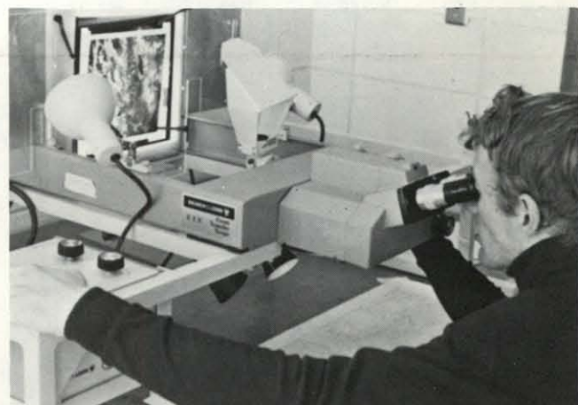
Fig. 2. On the Zoom Transfer Scope, illumination controls at the operator's left allow him to view either the LANDSAT image (on the vertical stage), or the map, or both at once. Scale, orientation and stretch controls at his right permit matching of the two images.
