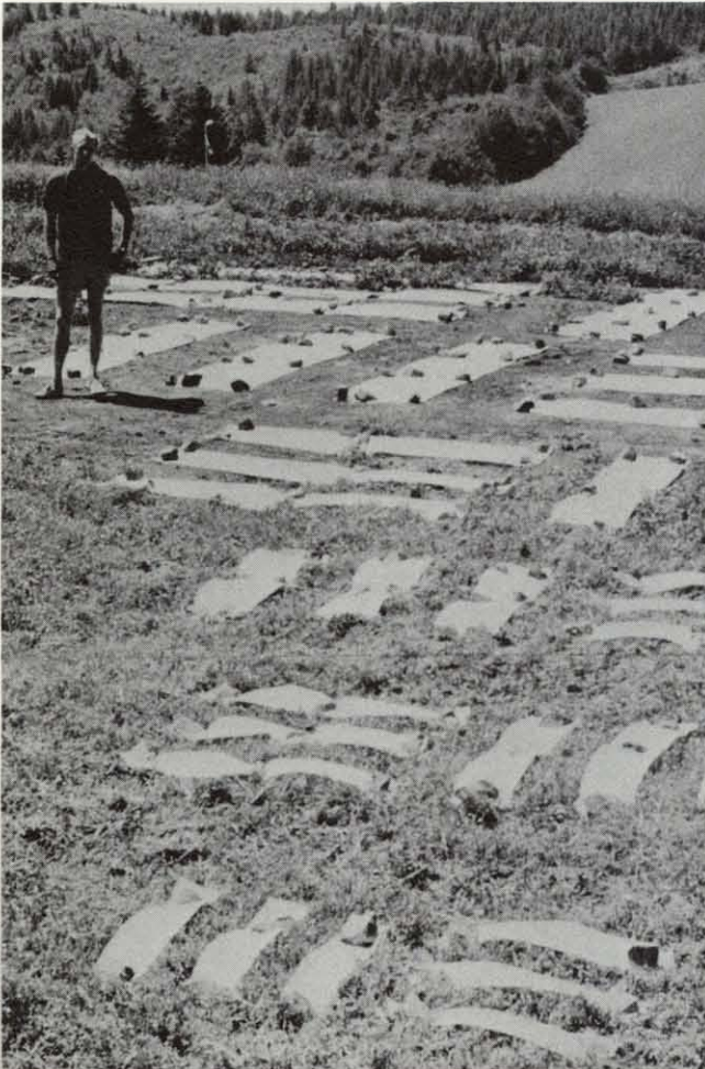
Figure 2. Seven target arrays were constructed, maintained in the field for a week, and removed. Damage from weather and domestic animals was repaired before each U-2 flight. Labor costs were about $900; materials about $300.
