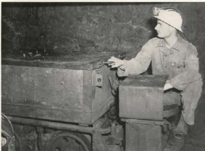
BRUCE WORMALD operates the miner's Cadillac, a battery-operated trammer.
