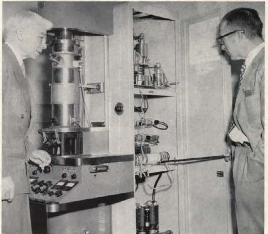
DR. WILLIAM CONE, right, and E. E. SPIKER test the new electron microscope that was donated this year to the University. Such a microscope is much more powerful than the ordinary optical variety, and promises much in the field of research.
