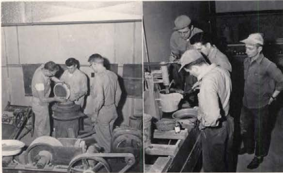
The students on the left are busy "making little ones out of big ones." On the right they are extracting sulphur from ore by way of a flotation process.
