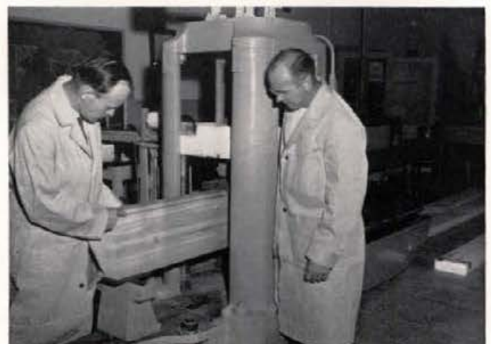
Professors John Howe and Arland Hofstrand testing the strength of a beam in wood utilization lab.
