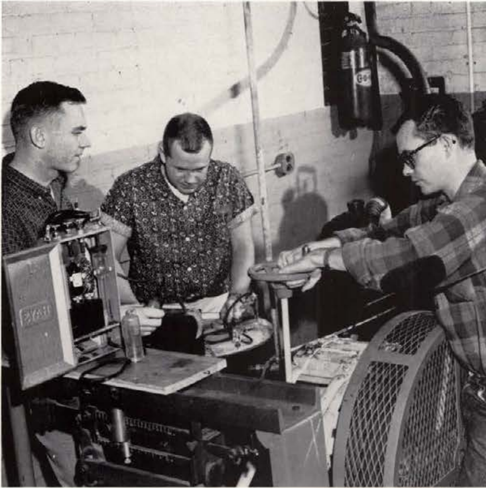
Dean Kohntopp, Ralph Brown, and Alan Ross are making a combustion analysis of an engine's exhaust gas.
