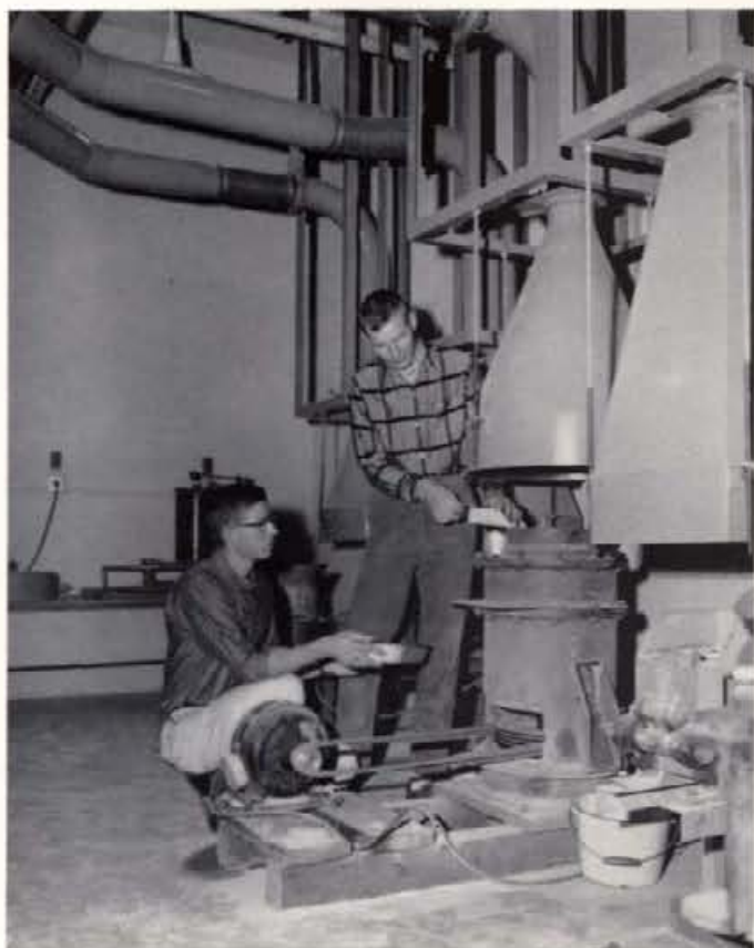
These two mining students are screening material in the process of determining the particular analysis of the different ore samples.
