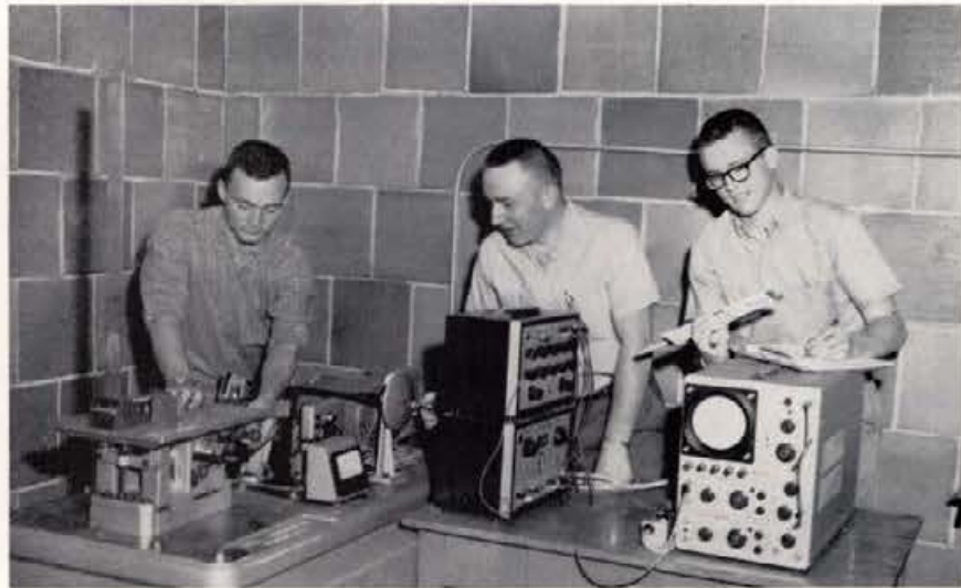
The effects of vibrations are studied by engineering students John Sackett, Don Dana, and Lance Whitehead, here working with a mechanical vibrating table.
