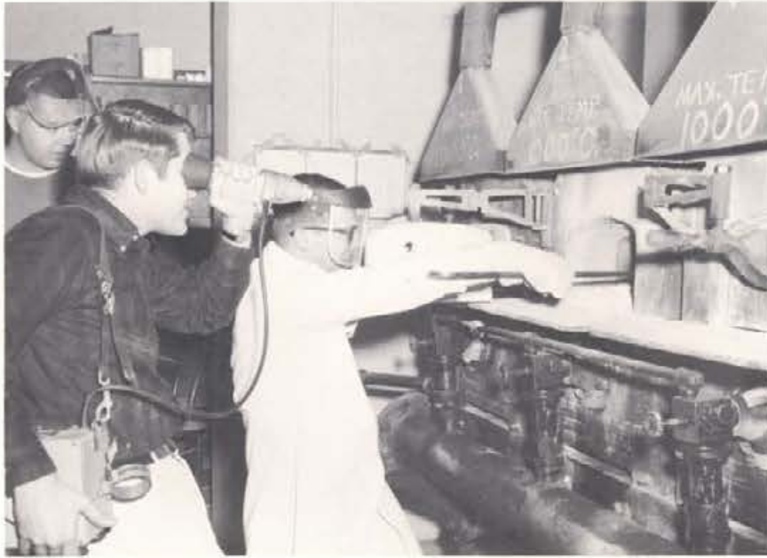
Curtis Carey, Richard Kunter, and Phil Helsley take a temperature reading of an oil-fired assay furnace with an optical pyrometer. The furnace is used to assay gold and silver.
