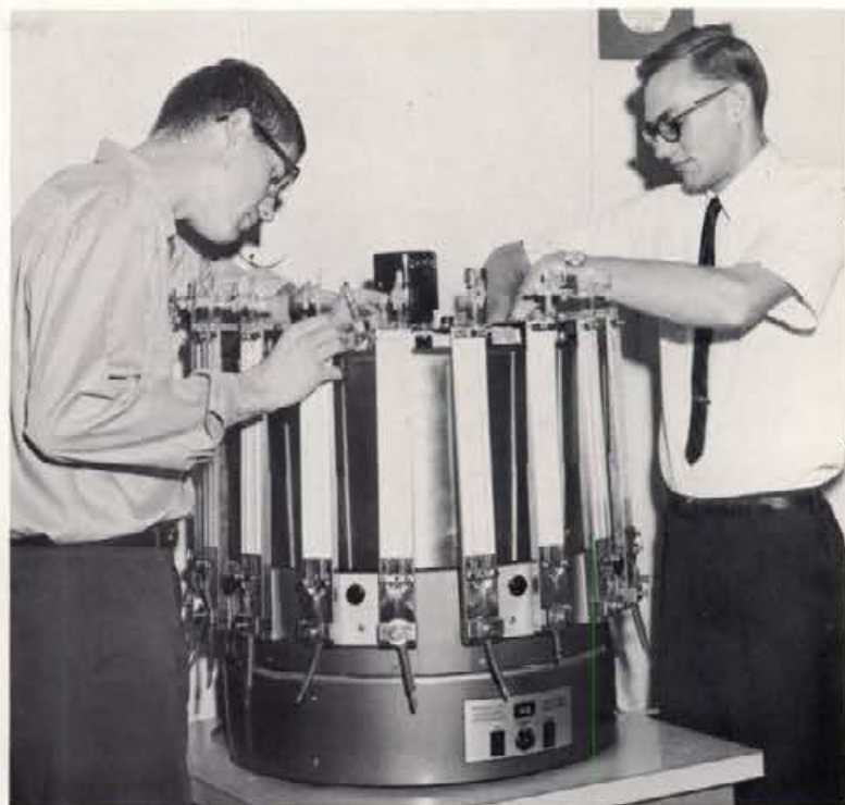
Dave Clarkson and Tom Richards work with the Warburg apparatus which is designed to measure respiratory gases and oxygen utilization.
