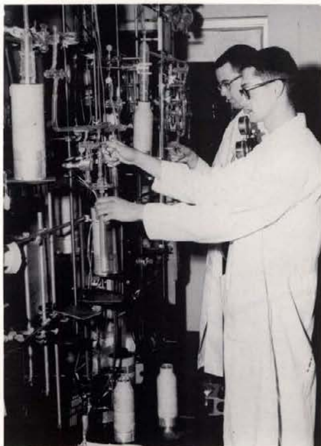
George Fraser and Dan Babb demonstrate the vacuum-line techniques used to synthesize new fluorine-containing compounds.
