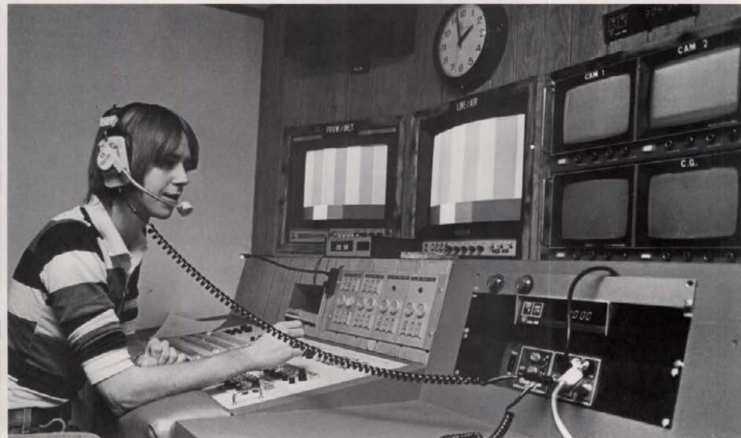
TECHNICAL DIRECTOR Dave Hanson operates the production switcher in the director's booth.
