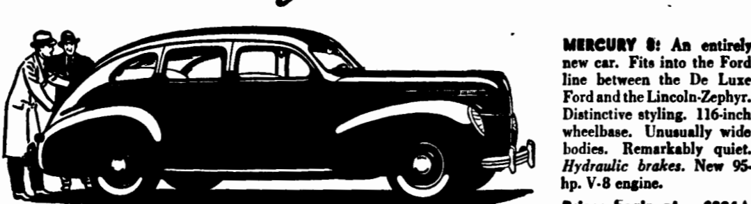
The Mercury 8 is an entirely new car. Fits into the Ford line between the De Luxe Ford and the Lincoln-Zephyr. Distinctive styling. 116-inch wheelbase. Unusually high bodies. Remarkably quiet. Hydraulic brakes. New 95-hp. V-8 engine. Prices begin at...$694*
