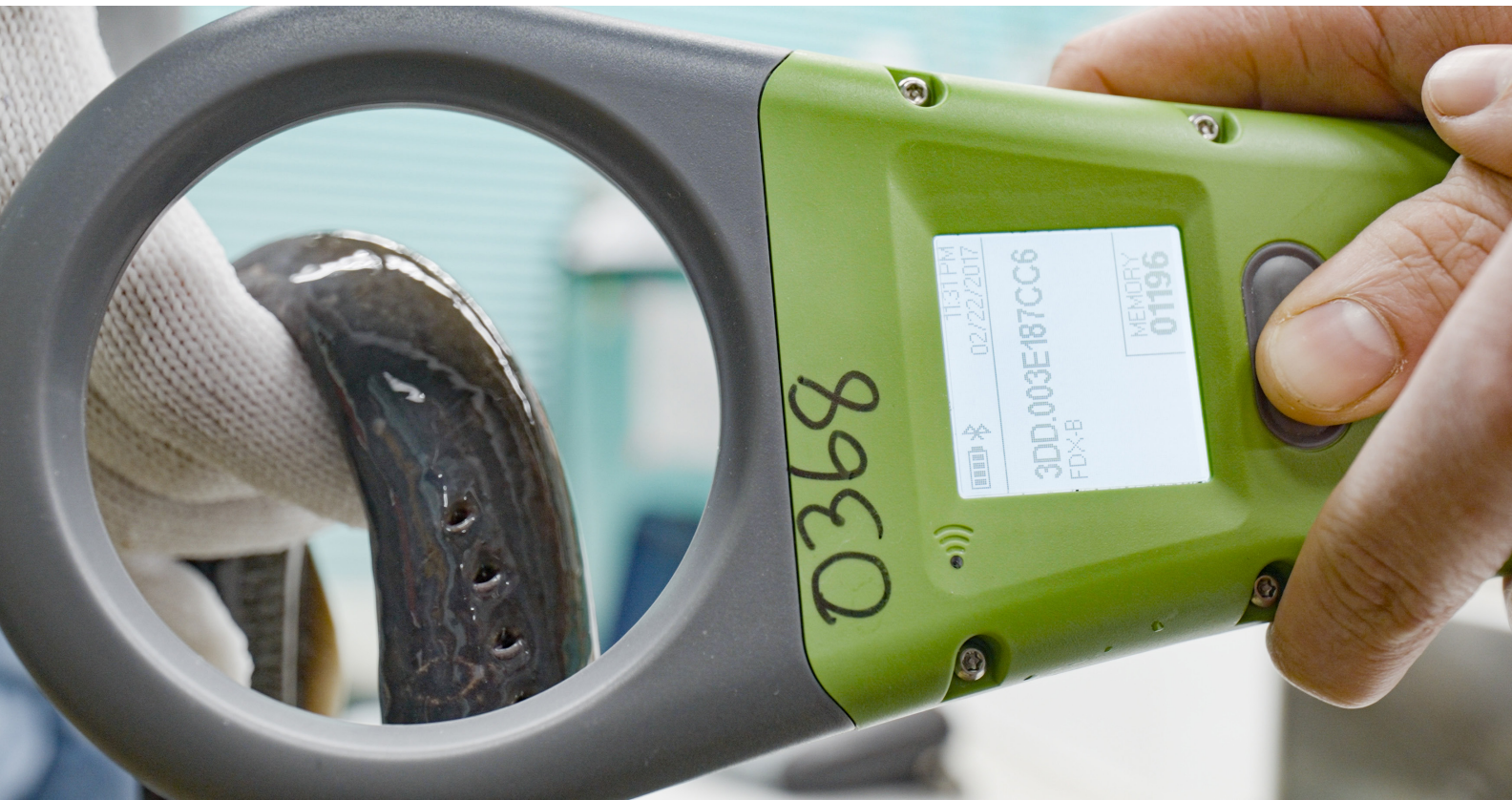
Researchers identify each lamprey using a handheld device that recognizes passive integrated transponder tags embedded in the fish.
