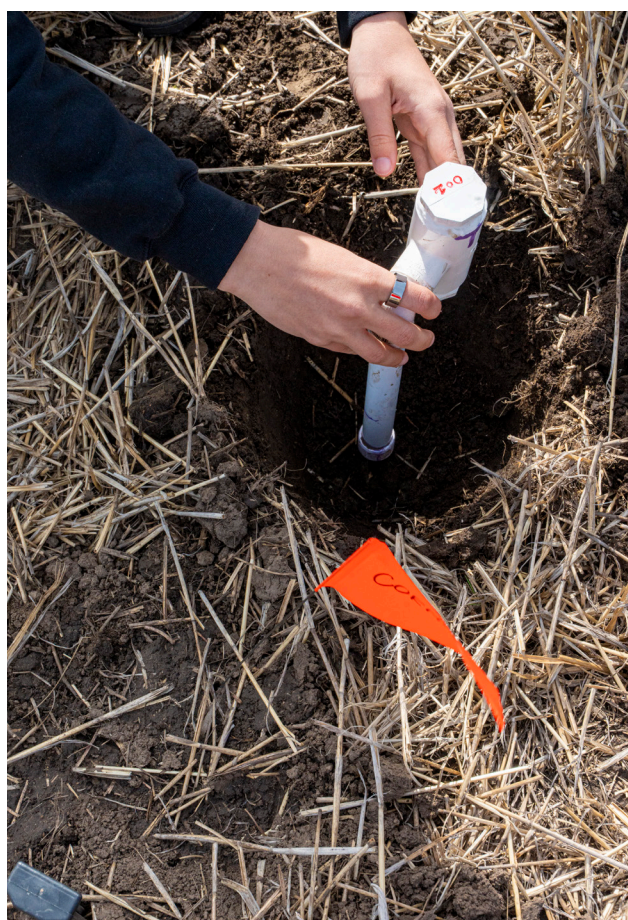
Nearly 300 soil sensors were installed south of Moscow to monitor moisture across varying slopes.
