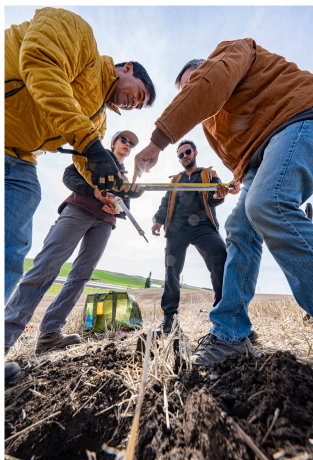
The research team prepares to install a soil moisture sensor deep in a wheat field at U of I's Kambitsch Farm near Genesee.
