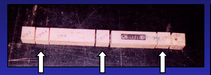
Compression tests are performed at three locations on the mineral soil stakes and one location in the middle of the surface stakes.
