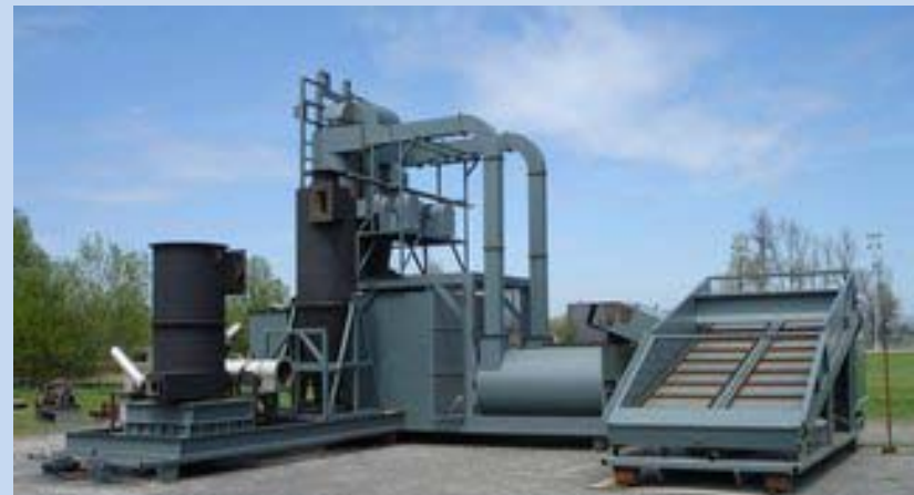
ABRI 50 ton/day mobile fast pyrolysis unit
