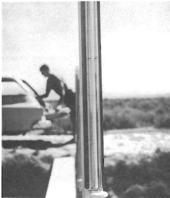
B. Double tube mercury manometer for tensiometer readout. FIGURE 9 TENSIO METER TIP AND MANOMETER FIELD TENSIO METER STUDIES NORTHSIDE PUMPING CANAL.
