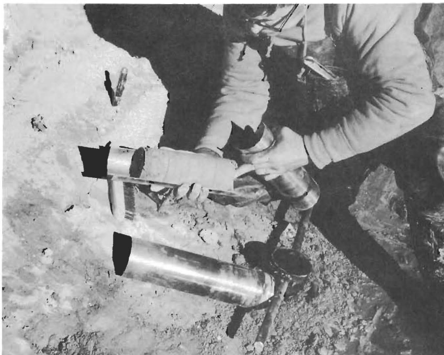
B. Sampler in use on silt loam soil. FIGURE 19 UNDISTURBED CORE SAMPLER INVESTIGATION OF IMPEDING SILT LAYER NORTHSIDE PUMPING CANAL
