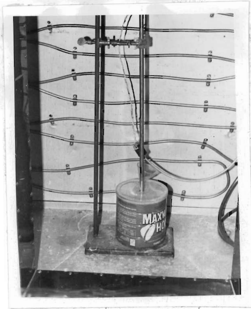
Figure 32. For testing of Prototype II, the soil sample occupied a 3-pound coffee can whose lid was sealed with the exception of the funnel tube through which water was added. The sample temperature was varied to sub-zero by a large upright Amana freezer. The freezer shelves were removed and the cooling coils were moved to the freezer's back wall.
