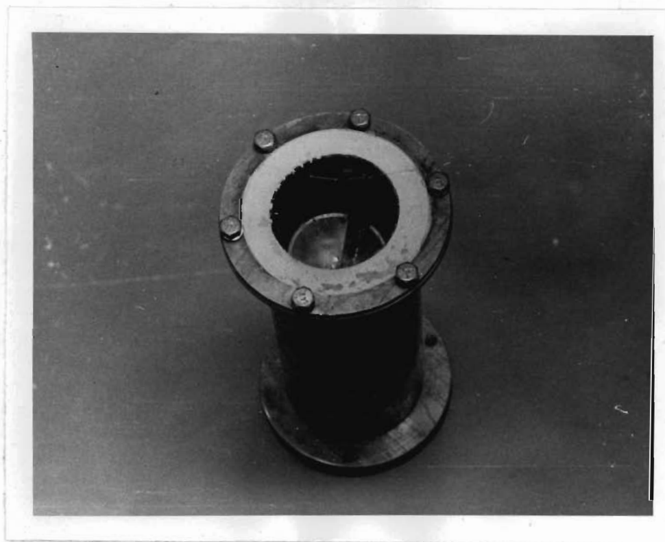
Figure 10. Assembled IR moisture detector, bottom view, showing window through which measurements are taken.
