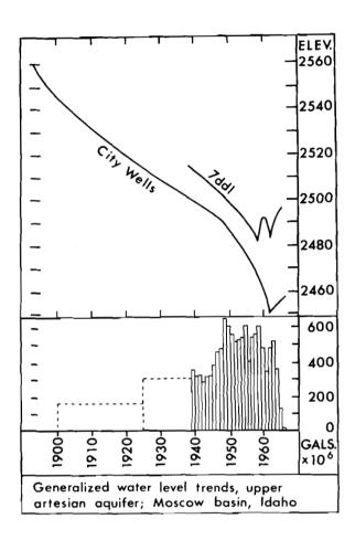
Figure 3. Water level trends (generalized) and water pumped, 1896-1965, Moscow basin, Latah County, Idaho.
