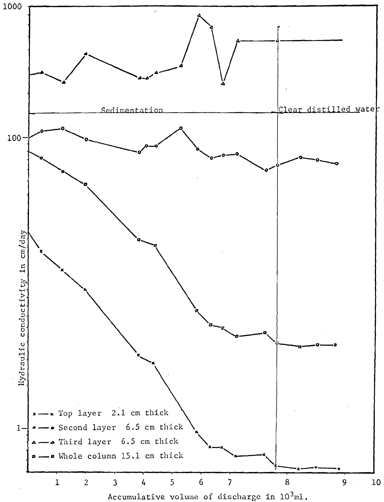
Figure 14. Variation of hydraulic conductivity with accumulated volume of discharge in sedimentation Series I Run A
