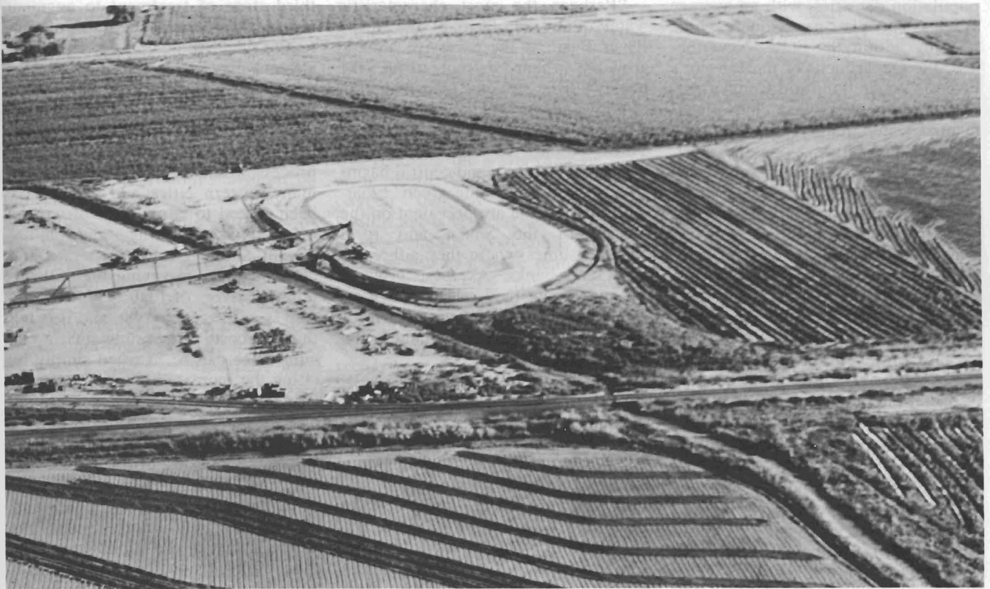
This aerial view of the fields shows the corrugates which are used to help spread the canning factory wastewater. The eight-foot-high stick in the middle of the corn field shows what irrigating with canning factory wastewater can do.
