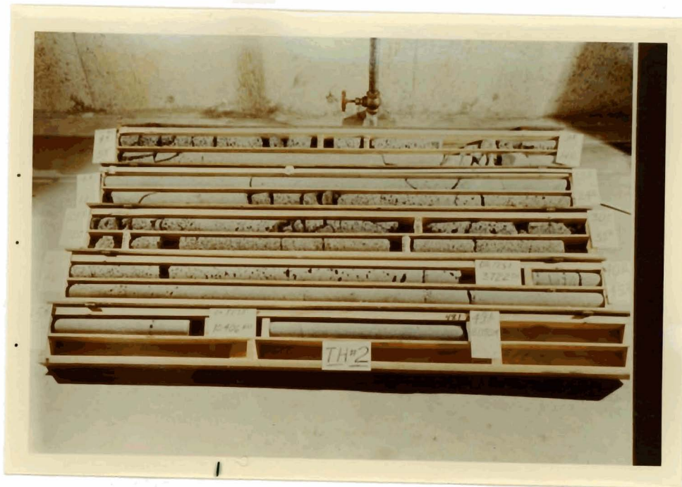
Figure 12. Vesicular structure in upper part of basalt, National Reactor Testing Station (not in study area).
