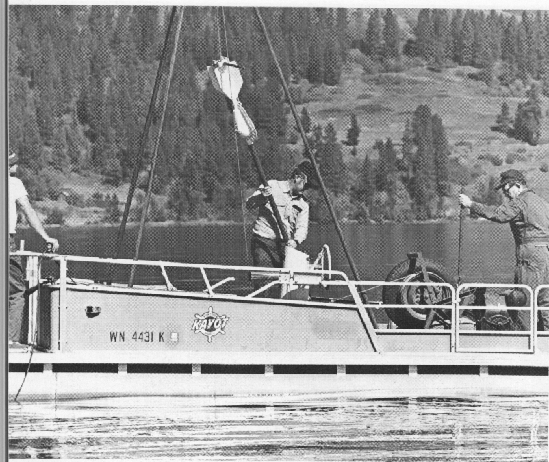
Above: A barge-mounted piston corer is used to bring up samples of bottom muds for later laboratory analyses to determine metal content. From left to right, WSU sanitary engineering section members Pat Syms, William Funk, and civil engineering department member Leo Cunningham. Below: Water samples are taken at a number of Coeur d'Alene Lake locations as well as in the Spokane River. At left, WSU sanitary engineer Richard Condit. At right, student Neil Thompson. To the right: Some water quality measurements are made on-board as soon as the sample has been collected. Richard Condit records his finding.
