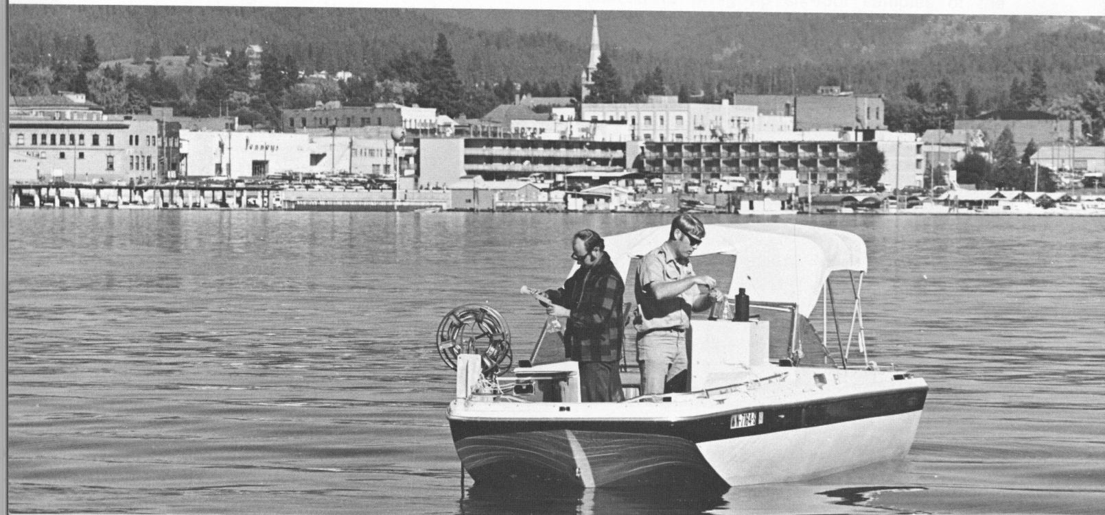
Above: A barge-mounted piston corer is used to bring up samples of bottom muds for later laboratory analyses to determine metal content. From left to right, WSU sanitary engineering section members Pat Syms, William Funk, and civil engineering department member Leo Cunningham. Below: Water samples are taken at a number of Coeur d'Alene Lake locations as well as in the Spokane River. At left, WSU sanitary engineer Richard Condit. At right, student Neil Thompson. To the right: Some water quality measurements are made on-board as soon as the sample has been collected. Richard Condit records his finding.
