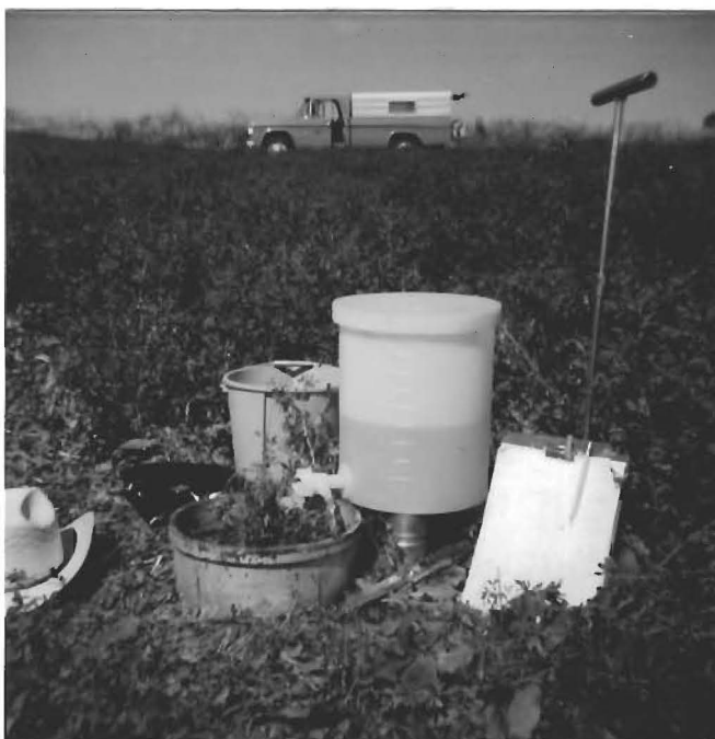
Figure 11. Ring infiltrometer in place during infiltration test.
