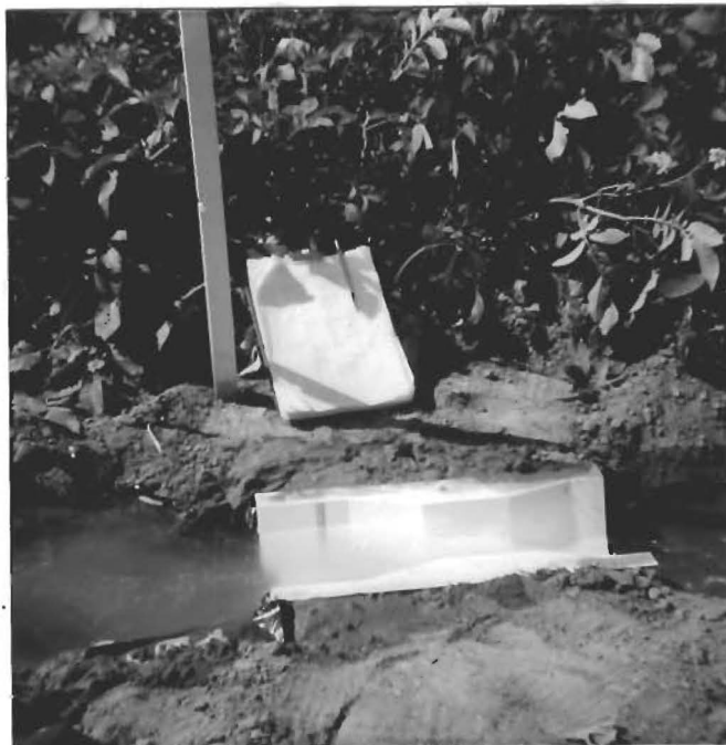
Figure 13. Trapezoidal flume installed at downstream station of furrow.
