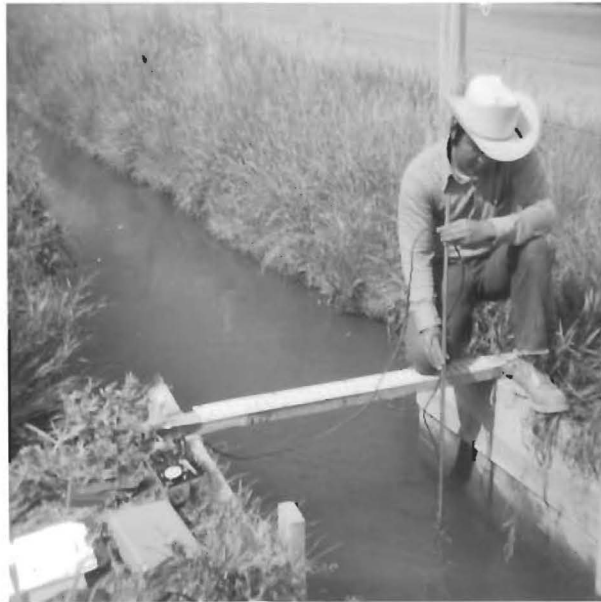
Figure 8. Measuring stream flow in an irrigation lateral.
