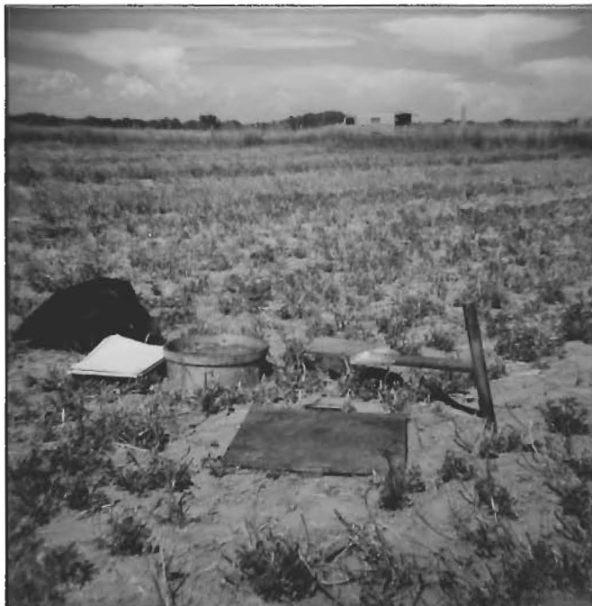
Figure 10. Ring infiltrometer with driving hammer and plate.
