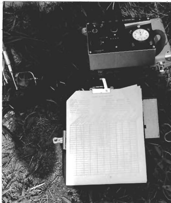
Figure 9. Current meter and counter used in stream-flow measurement.
