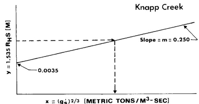
Fig. 11. Unit dry bedload transport capacity of Knapp Creek, as predicted by the Meyer-Peter, Muller equation.
