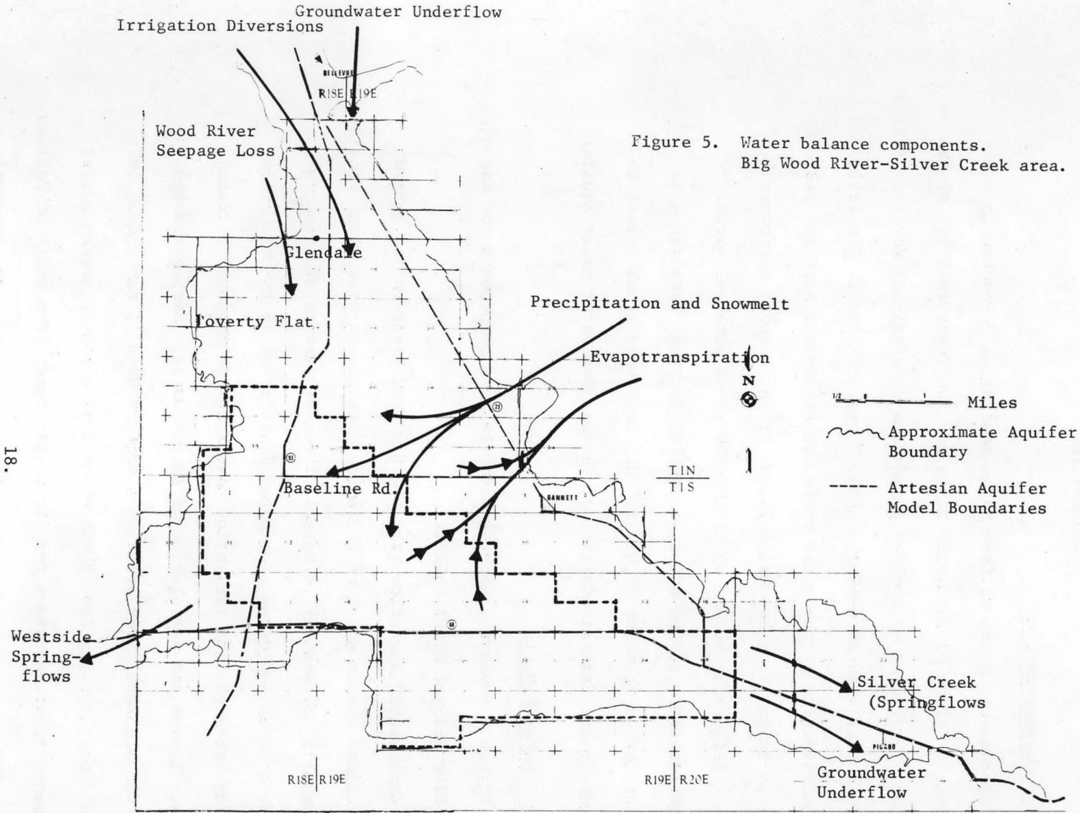
Figure 5. Water balance components. Big Wood River-Silver Creek area.
