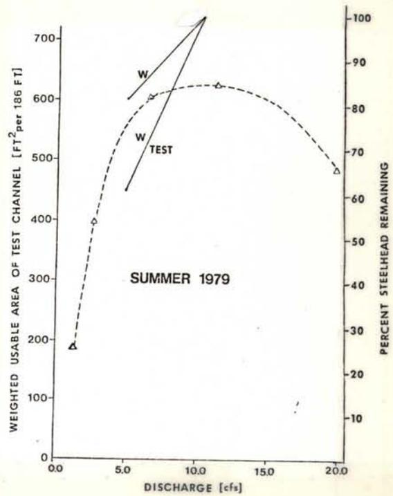
Figure 73. Comparison of weighted useable area (dashed line) and response of juvenile rainbow-steelhead trout populations to discharge in test and control channels, Instream Flow Research Facilities, Grande Ronde River, Wallowa County, Oregon, fall 1978, and summer 1979.
