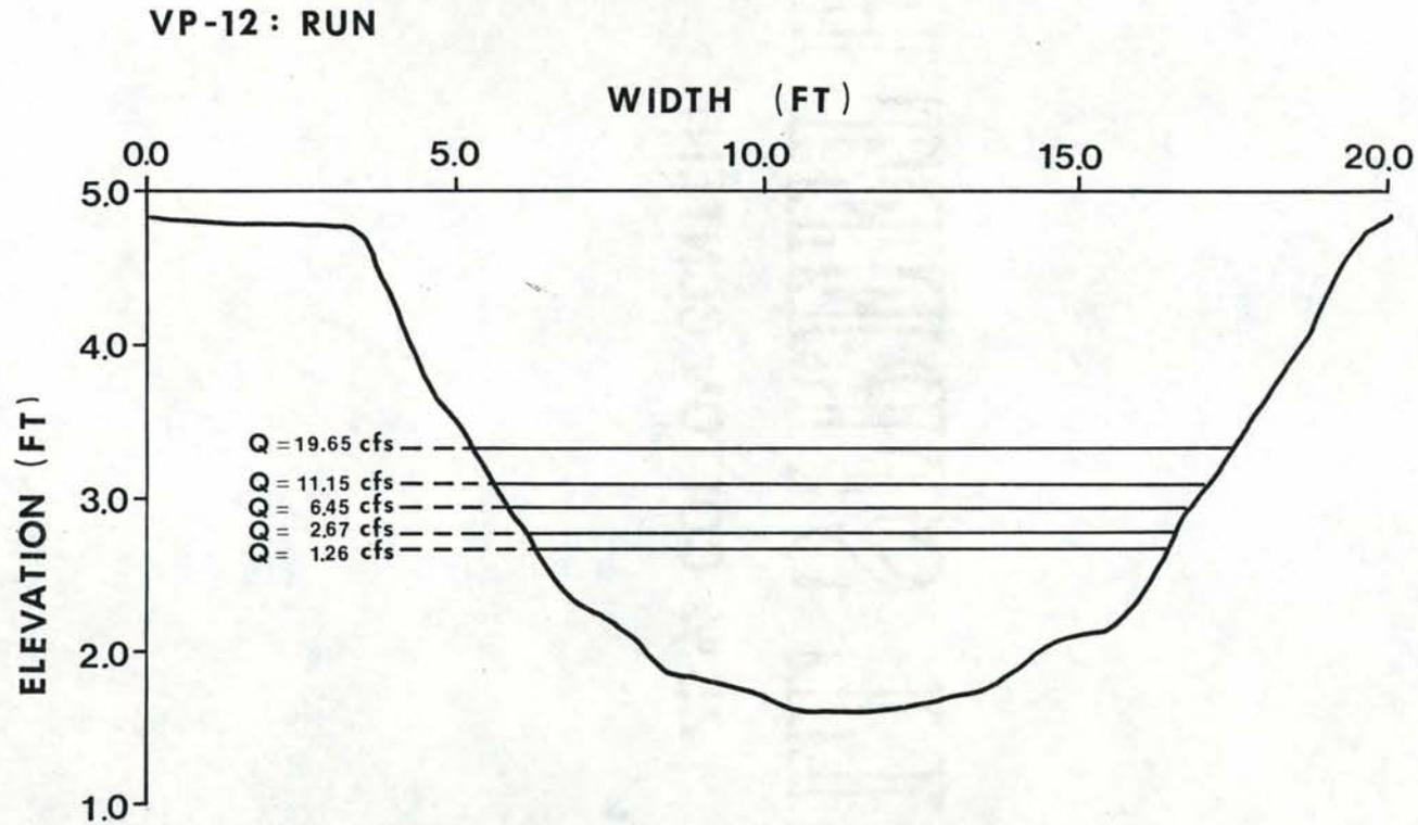
Figure 54. Typical cross sectional shape of a run transect at five test flows, west channel Troy Instream Flow Research Facilities, Grande Ronde River, Wallowa County, Oregon, fall 1978.
