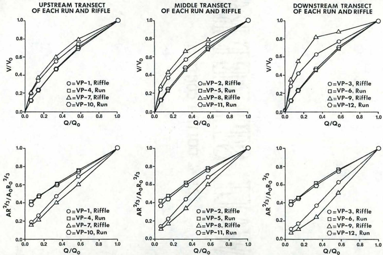
Figure 59. Velocity ( $V$ ) and section factor ( $AR^{2/3}$ ) versus discharge ( $Q$ ) for non-transitional stream reach, west channel, Troy Instream Flow Research Facilities, Grande Ronde River, Wallowa County, Oregon, fall 1978.
