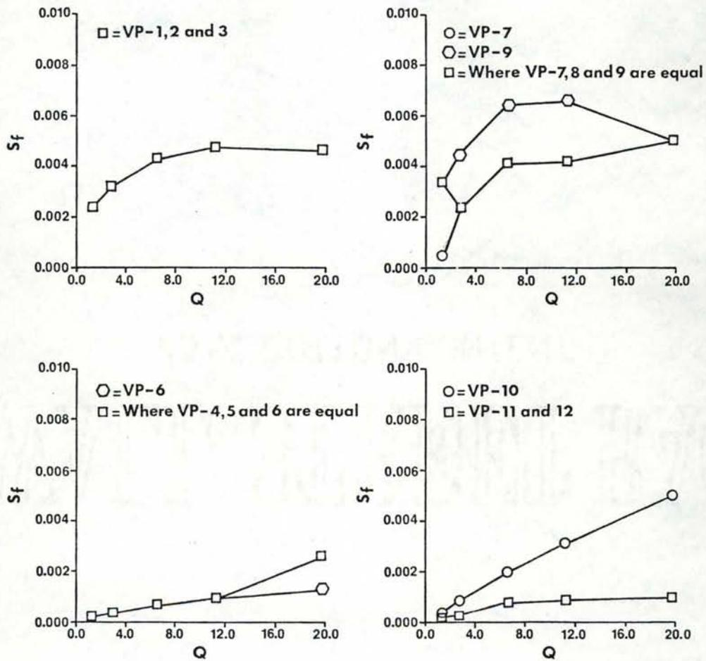
Figure 61. Relationship between the energy slope ( $S_f$ ) and discharge ( $Q$ ) in riffle and run reaches, west channel, Troy Instream Flow Research Facilities, Grande Ronde River, Wallowa County, Oregon, fall 1978.
