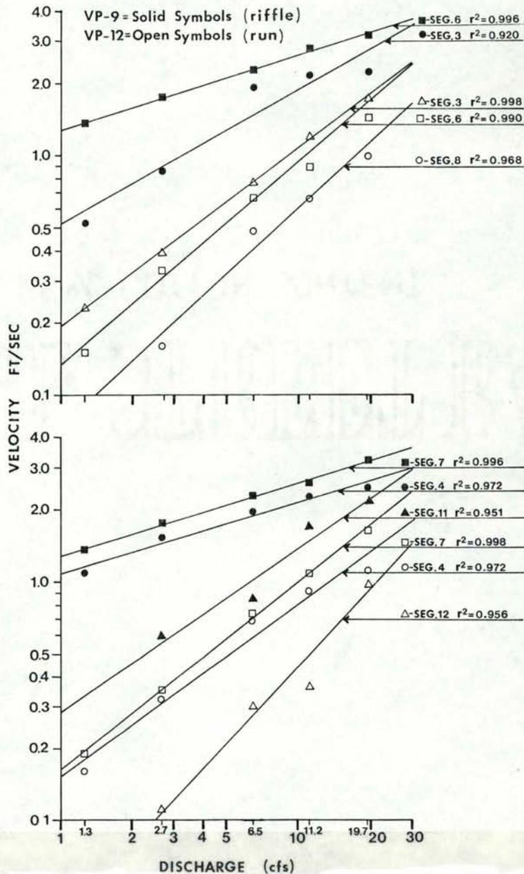
Figure 68. Log-log plot of measured average segment velocities versus total discharge through a cross section used to evaluate the equation  $v_x = a Q^{bx}$  in the IFG-4 hydraulic simulation model, west channel, Troy In-stream Flow Research Facilities, Grande Ronde River, Wallowa County, Oregon, fall 1978.
