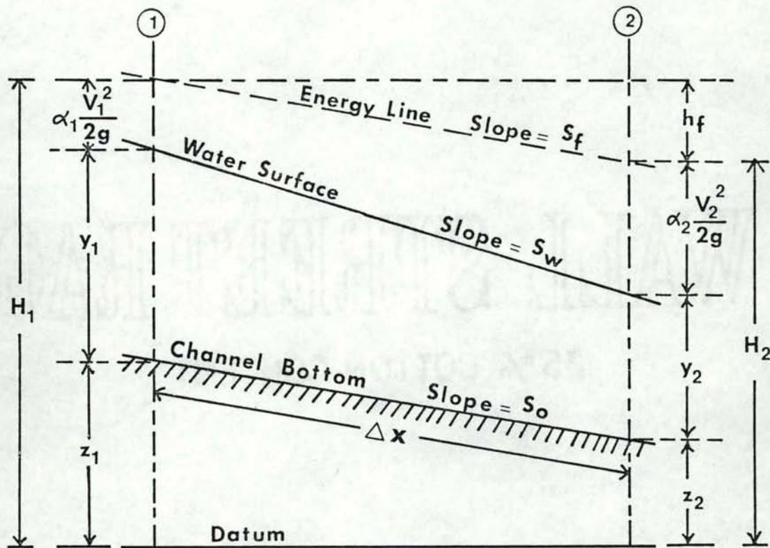
Figure 46. Energy in gradually varied open channel flow (from Chow 1959).
