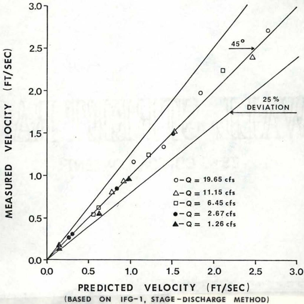
Figure 62. Comparison of predicted with measured average cross sectional velocities using the IFG-1 model, stage-discharge option; calibrated with stage-discharge pairs at 11.15, 6.45, and 2.67 ft<sup>3</sup>/s, west channel, Troy Instream Flow Research Facilities, Grande Ronde River, Wallowa County, Oregon, fall 1978.
