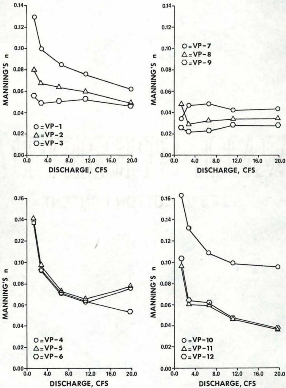
Figure 60. Relationship between Manning's roughness coefficient (n) and discharge (Q) in riffle and run reaches, west channel, Troy Instream Flow Research Facilities, Grande Ronde River, Wallowa County, Oregon, fall 1978.
