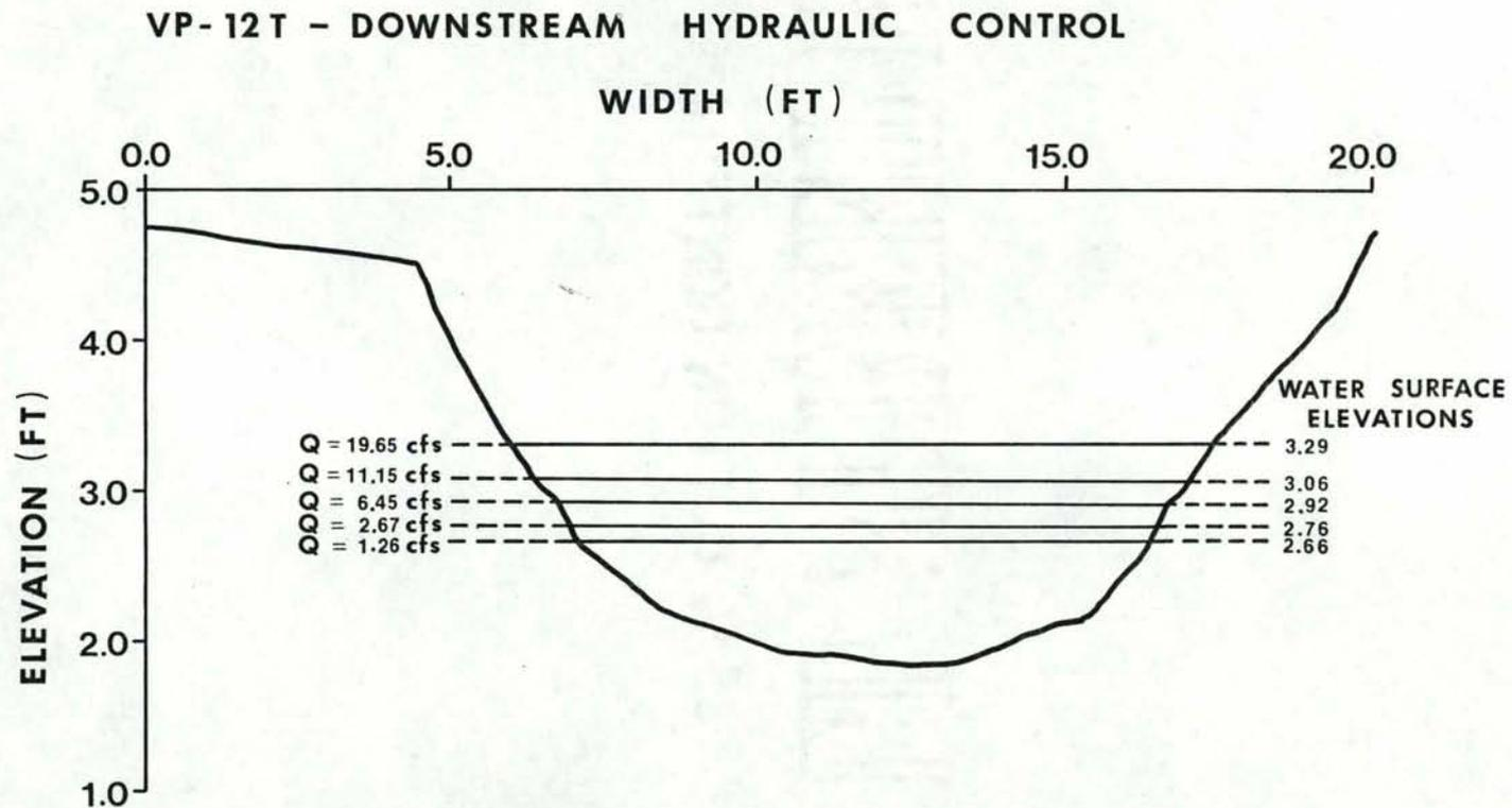
Figure 50. Cross section of most downstream VP (12T) transect showing five test flows with associated water surface elevations, west channel, Troy Instream Flow Research Facilities, Grande Ronde River, Wallowa County, Oregon, fall 1978.
