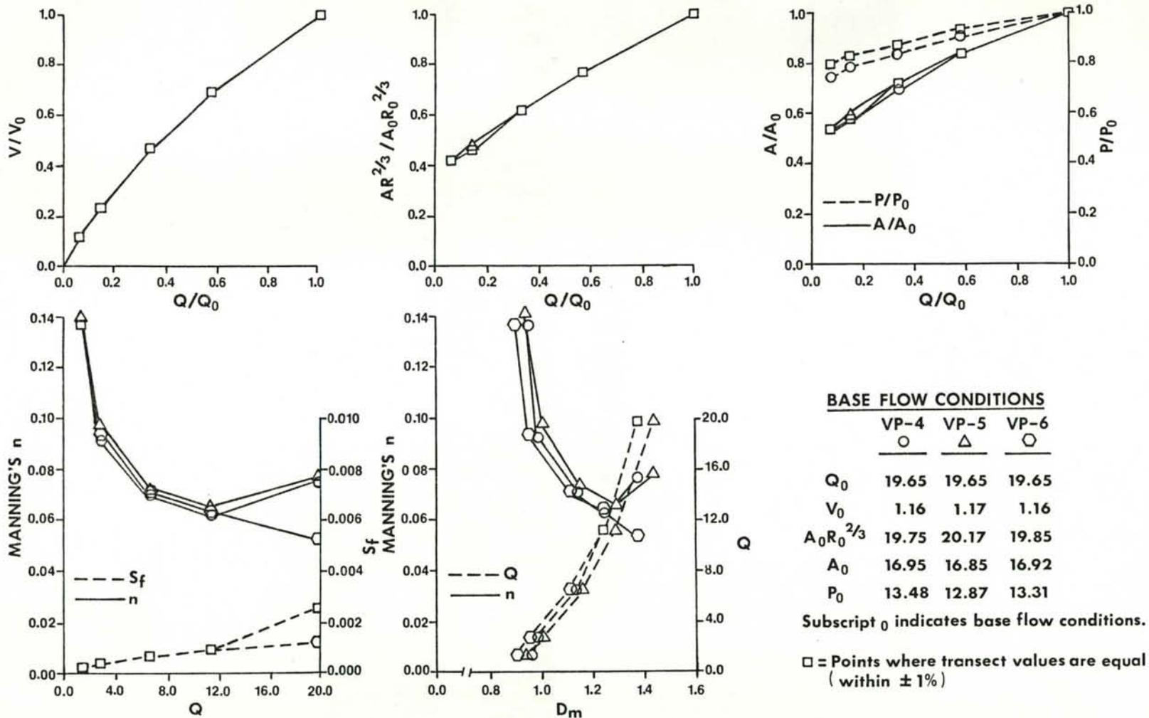
Figure 52. Stream flow characteristics; discharge ( $Q$ ), average cross section velocity ( $V$ ), section factor ( $AR^{2/3}$ ), area ( $A$ ), wetted perimeter ( $P$ ), mean depth ( $D_m$ ), Manning's roughness coefficient ( $n$ ), and energy slope ( $S_f$ ), of VP-4, 5 and 6, the upstream run, west channel, Troy Instream Flow Research Facilities, Grande Ronde River, Wallowa County, Oregon, fall 1978.
