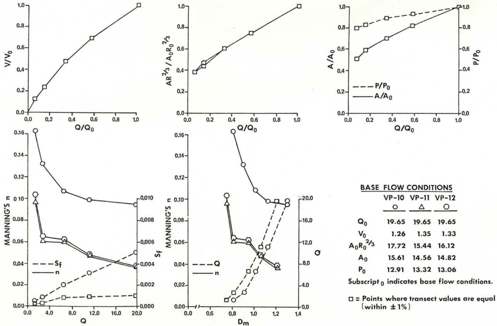
Figure 53. Stream flow characteristics; discharge ( $Q$ ), average cross section velocity ( $V$ ), section factor ( $AR^{2/3}$ ), area ( $A$ ), wetted perimeter ( $P$ ), mean depth ( $D_m$ ), Manning's roughness coefficient ( $n$ ), and energy slope ( $S_f$ ), of VP-10, 11 and 12, the downstream run, west channel, Troy Instream Flow Research Facilities, Grande Ronde River, Wallowa County, Oregon, fall 1978.
