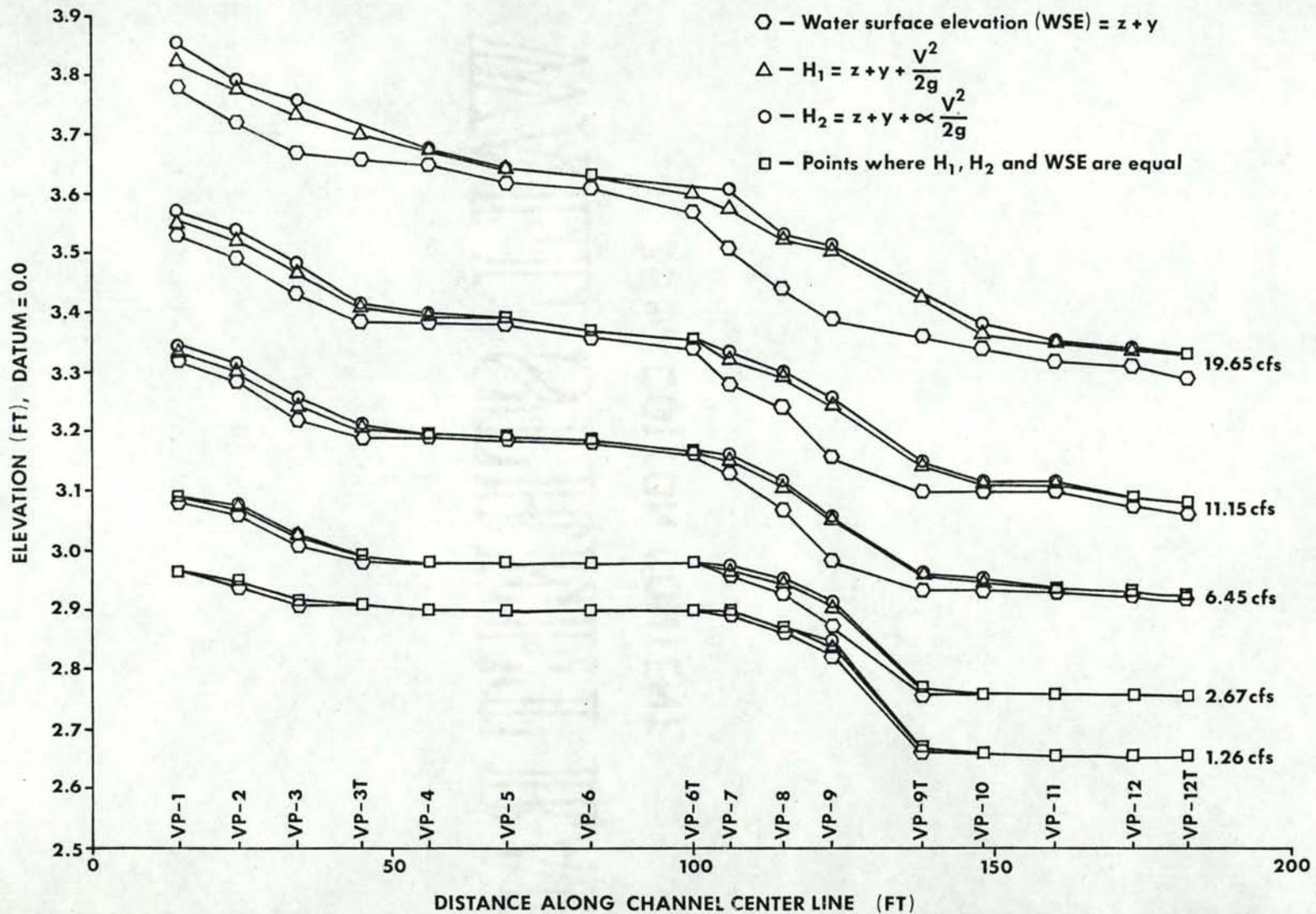
Figure 51. Comparison of the energy grade lines ( $H_1$  and  $H_2$ ) and hydraulic grade line (WSE) at the five experimental flows, west channel, Troy Instream Flow Research Facilities, Grande Ronde River, Wallowa County, Oregon, fall 1978.
