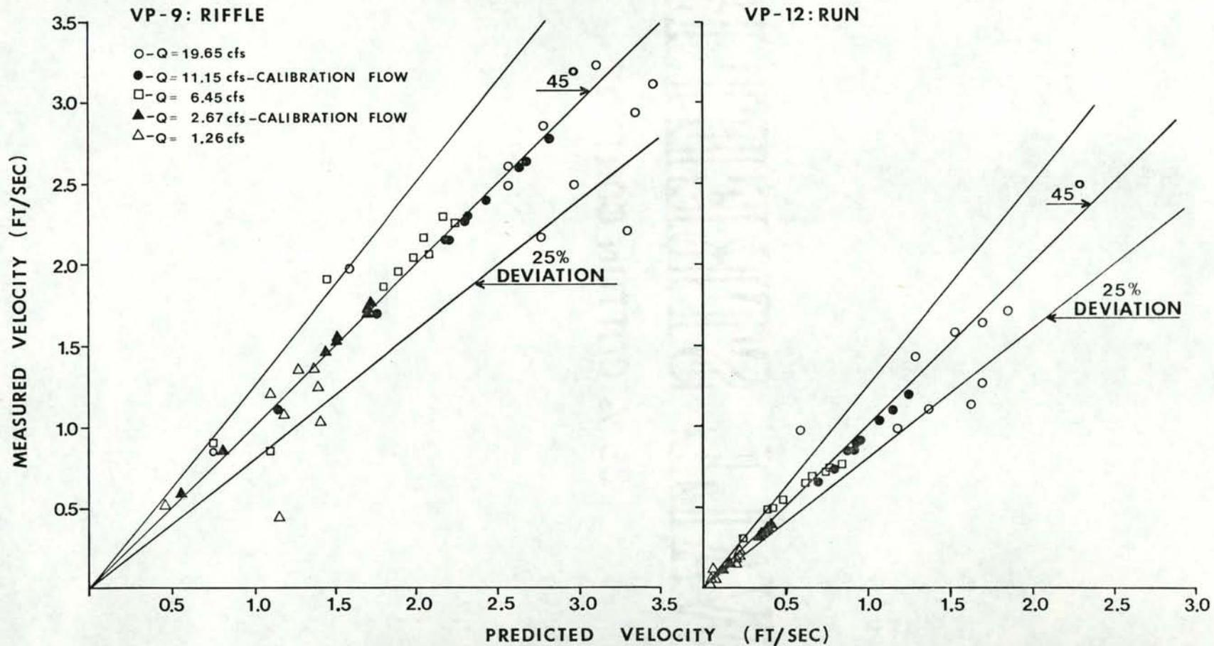
Figure 69. Comparison of predicted average segment velocities with measured velocities using IFG-4 model calibrated at 11.15, 6.45, and 2.67  $\text{ft}^3/\text{s}$  for a riffle (VP-9) and a run (VP-12) transect, west channel, Troy Instream Flow Research Facilities, Grande Ronde River, Wallowa County, Oregon, fall 1978.
