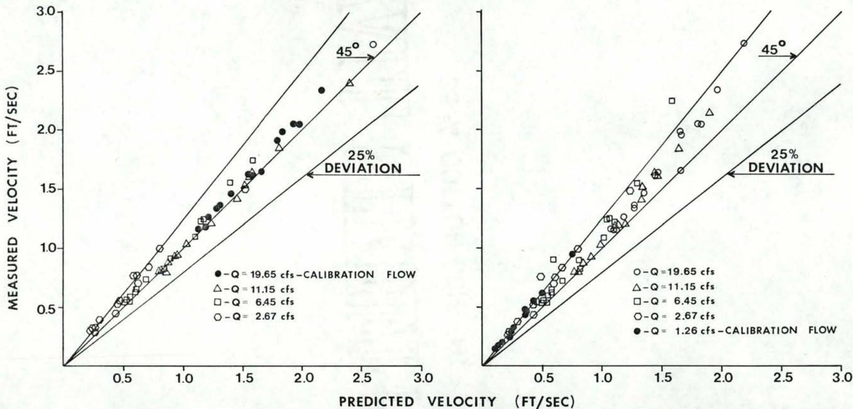
Figure 65. Comparison of predicted and measured average cross section velocities using the WSP model calibrated at  $19.65 \text{ ft}^3/\text{s}$  and  $1.26 \text{ ft}^3/\text{s}$ , west channel, Troy Instream Flow Research Facilities, Grande Ronde River, Wallowa County, Oregon, fall 1978.
