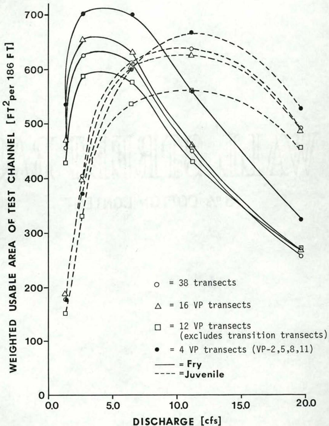
Figure 72. Changes in weighted usable area, for fry and juvenile rainbow-steelhead trout (*Salmo gairdneri*), as a result of reducing the number of transects used to describe the hydraulics of a stream reach, west channel, Troy Instream Flow Research Facilities, Grande Ronde River, Wallowa County, Oregon, fall 1978.
