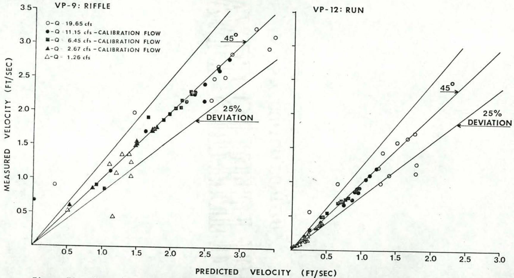
Figure 70. Comparison of predicted average segment velocities with measured velocities using IFG-4 model calibrated at 11.15 and 2.67  $\text{ft}^3/\text{s}$  for a riffle (VP-9) and a run (VP-12) transect, west channel, Troy Instream Flow Research Facilities, Grande Ronde River, Wallowa County, Oregon, fall 1978.
