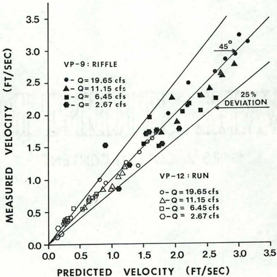
Figure 66. Comparison of predicted average segment velocities with measured velocities for a run transect (VP-12) and a riffle transect (VP-9) using the WSP hydraulic simulation model calibrated at 19.65 ft<sup>3</sup>/s with eight segments per transect, west channel, Troy Instream Flow Research Facilities, Grand Ronde River, Wallowa County, Oregon, fall 1978.
