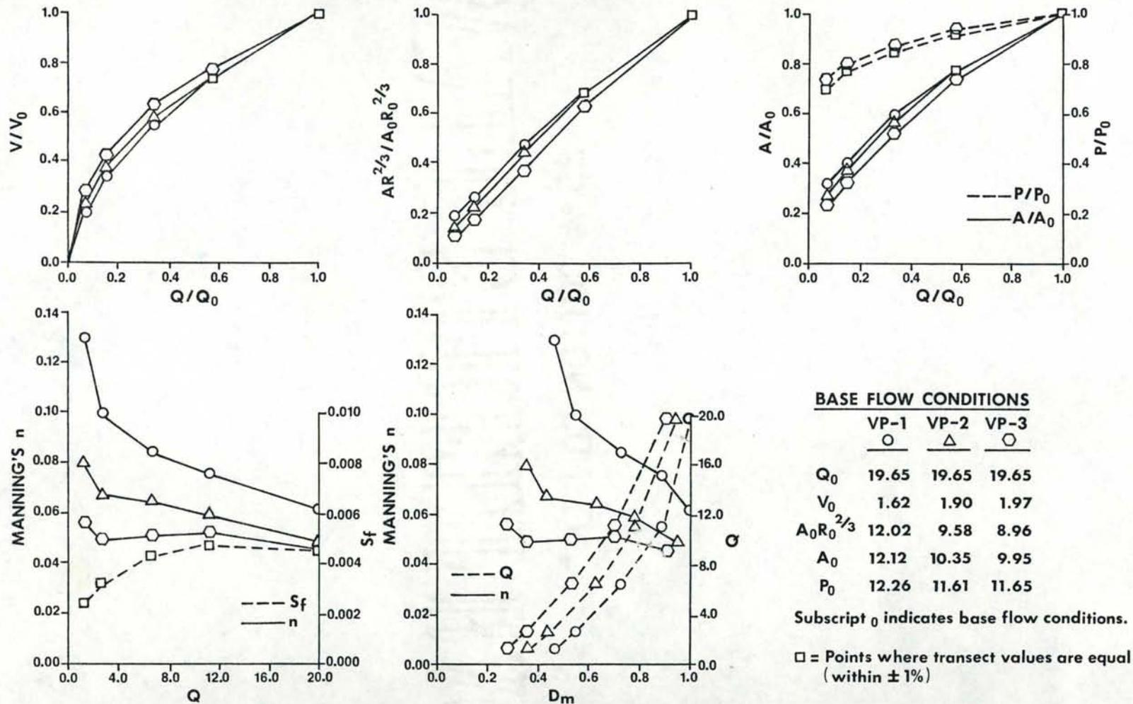
Figure 55. Stream flow characteristics; discharge ( $Q$ ), average cross section velocity ( $V$ ), section factor ( $AR^{2/3}$ ), area ( $A$ ), wetted perimeter ( $P$ ), mean depth ( $D_m$ ), Manning's roughness coefficient ( $n$ ), and energy slope ( $S_f$ ), of VP-1, 2 and 3, the upstream riffle, west channel, Troy Instream Flow Research Facilities, Grande Ronde River, Wallowa County, Oregon, fall 1978.
