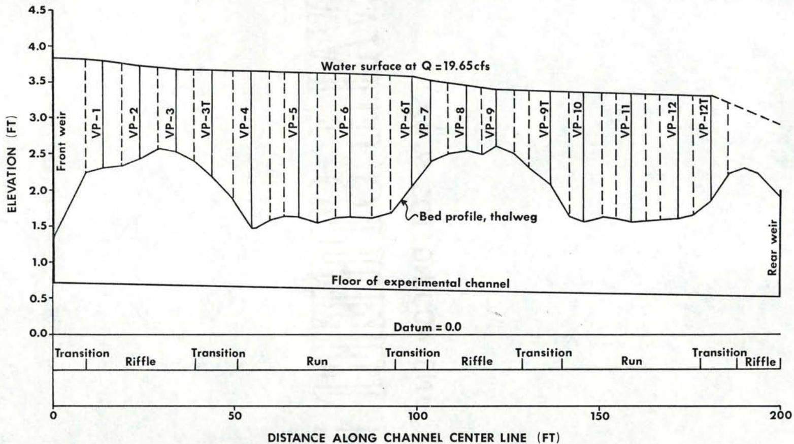
Figure 47. Profile of west channel at the thalweg with a flow of 19.65 ft<sup>3</sup>/s, showing locations of velocity profile transects, Troy Instream Flow Research Facilities, Grande Ronde River, Wallowa County, Oregon, fall 1978.
