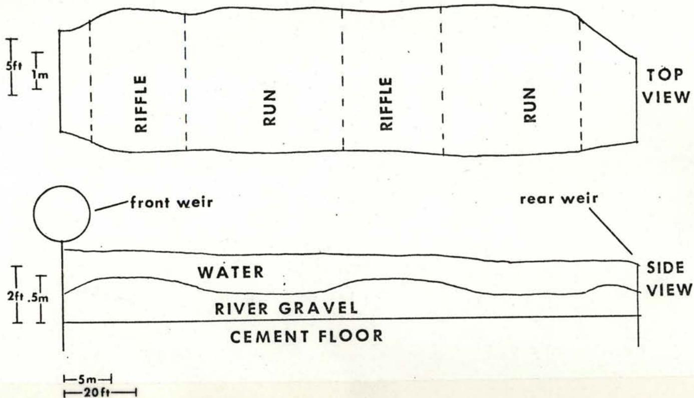
Figure 8. Schematic diagram of simulated stream channel of the Troy Instream Flow Research Facilities, Grande Ronde River, Wallowa County, Oregon. Water depths and widths represent a discharge of  $0.57 \text{ m}^3/\text{s}$  ( $20 \text{ ft}^3/\text{s}$ ).
