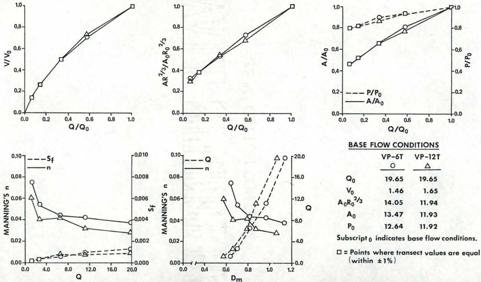
Figure 57. Stream flow characteristics; discharge ( $Q$ ), average cross section velocity ( $V$ ), section factor ( $AR^{2/3}$ ), area ( $A$ ), wetted perimeter ( $P$ ), mean depth ( $D_m$ ), Manning's roughness coefficient ( $n$ ), and energy slope ( $S_f$ ), of VP-6T, and 12T, the contracting transitions, west channel, Troy Instream Flow Research Facilities, Grande Ronde River, Wallowa County, Oregon, fall 1978.
