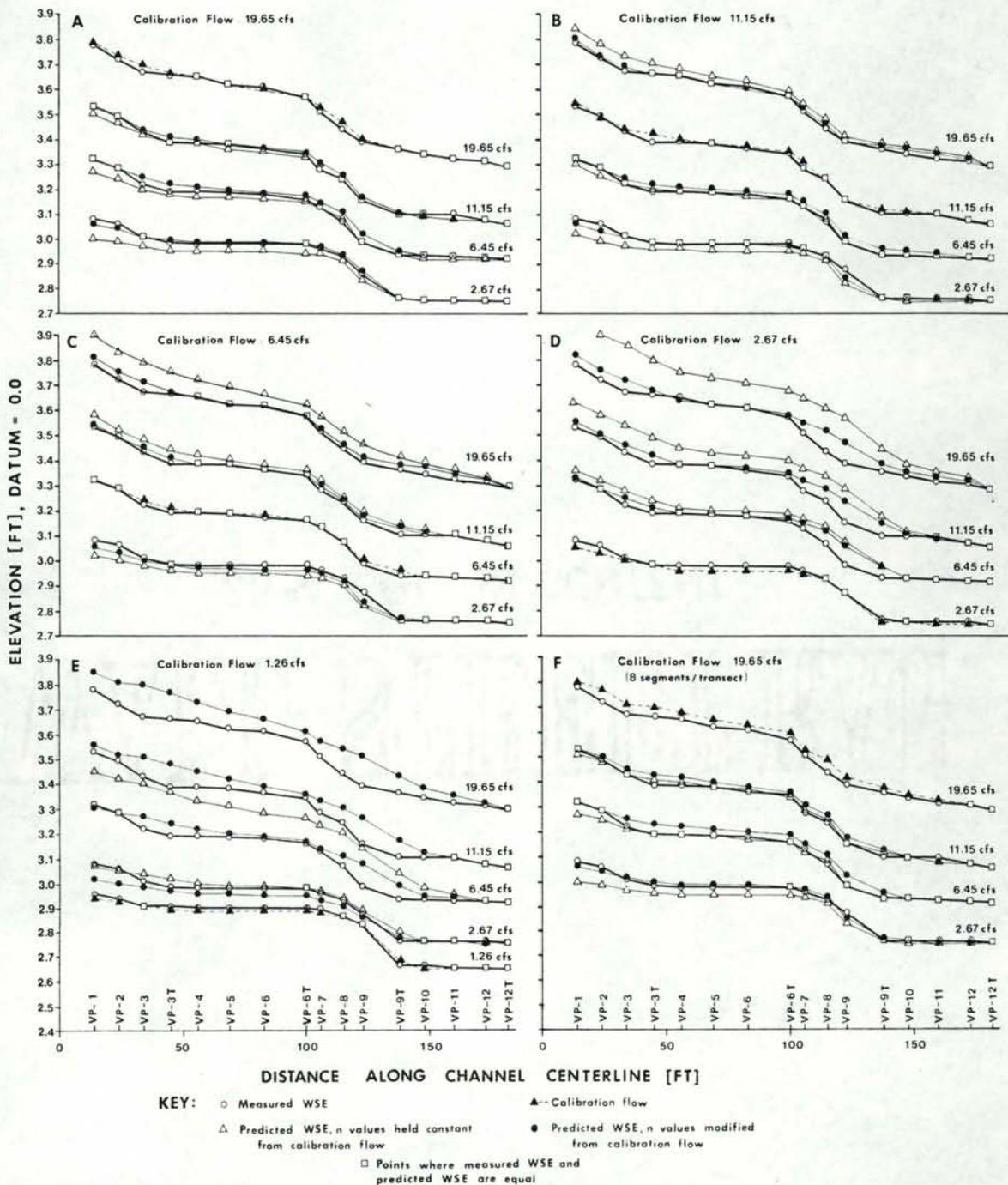
Figure 64. Comparison of measured and predicted water surface elevations using the WSP hydraulic simulation model calibrated at 19.65 ft<sup>3</sup>/s (A), 11.15 ft<sup>3</sup>/s (B), 6.45 ft<sup>3</sup>/s (C), 2.67 ft<sup>3</sup>/s (D), 1.26 ft<sup>3</sup>/s (E), and 19.65 ft<sup>3</sup>/s with transects divided into 8 segments (F), west channel, Troy Instream Flow Research Facilities, Grande Ronde River, Wallowa County, Oregon, fall 1978.
