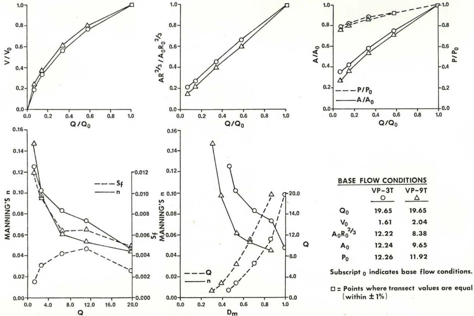
Figure 58. Stream flow characteristics; discharge (Q), average cross section velocity (V), section factor ( $AR^{2/3}$ ), area (A), wetted perimeter (P), mean depth ( $D_m$ ), Manning's roughness coefficient (n), and energy slope ( $S_f$ ), of VP-3T and 9T, the expanding transitions, west channel, Troy Instream Flow Research Facilities, Grande Ronde River, Wallowa County, Oregon, fall 1978.
