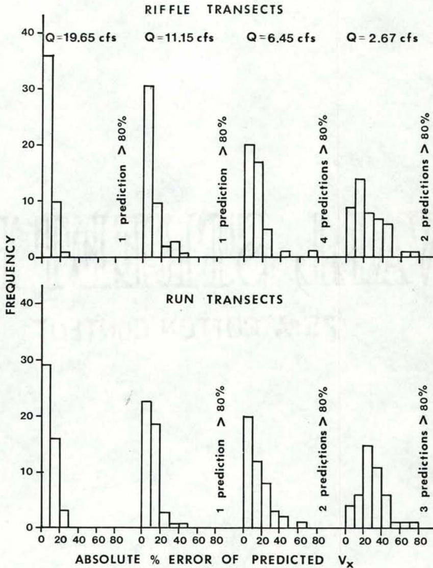
Figure 67. Magnitude in absolute percent error of measured versus predicted average segment velocities and frequency of error at 12 velocity profile transects with 8 segments per transect using the WSP hydraulic simulation model, west channel, Troy Instream Flow Research Facilities, Grande Ronde River, Wallowa County, Oregon, fall 1978.
