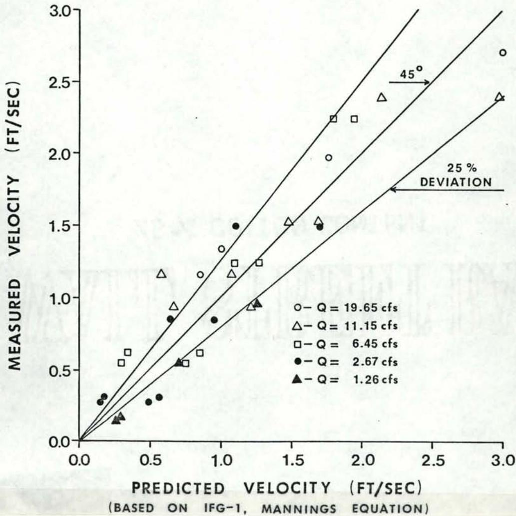
Figure 63. Comparison of predicted with measured average cross section velocities using the IFG-1 model, Manning's equation option, calibrations based upon Table 21 criteria, west channel, Troy Instream Flow Research Facilities, Grande Ronde River, Wallowa County, Oregon, fall 1978.
