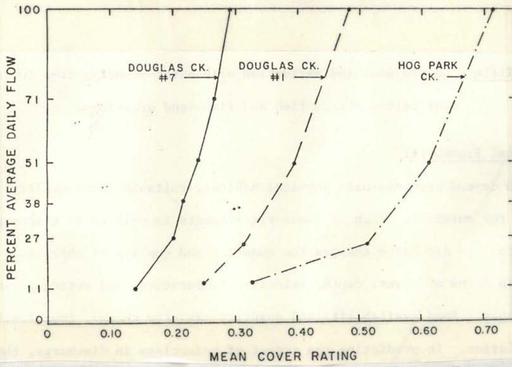
Figure 1. Changes observed in the mean trout cover rating as flow was reduced at the Douglas Creek No. 1, 7 and Hog Park Creek study areas (from Wesche 1974).
