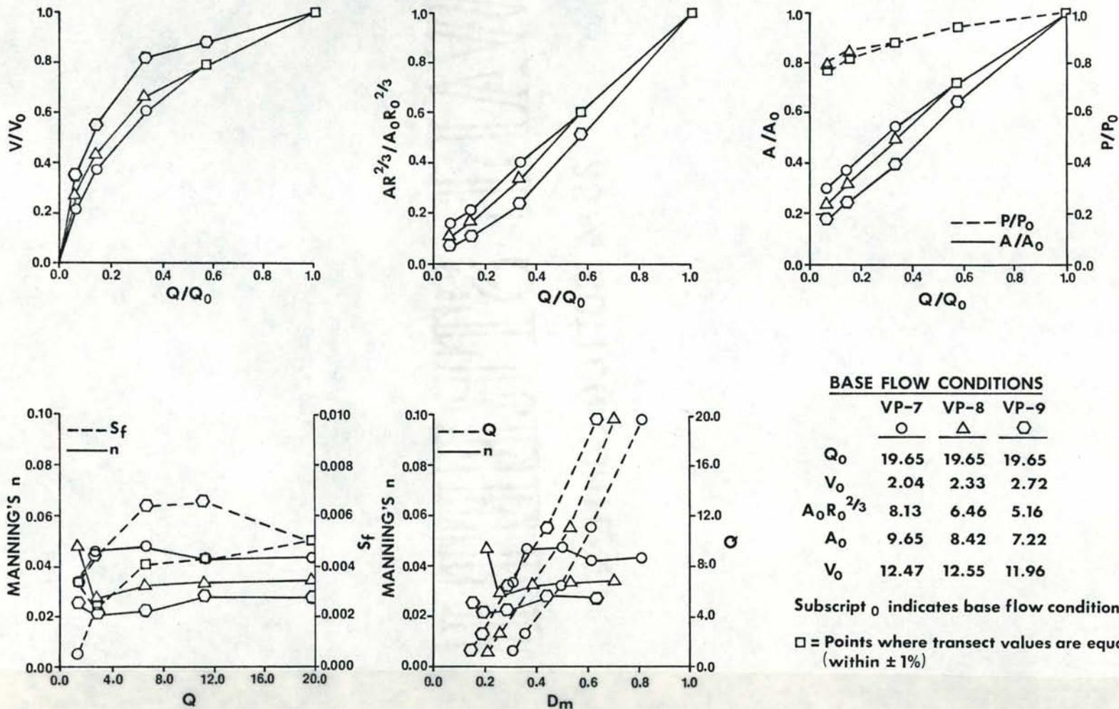
Figure 56. Stream flow characteristics; discharge ( $Q$ ), average cross section velocity ( $V$ ), section factor ( $AR^{2/3}$ ), area ( $A$ ), wetted perimeter ( $P$ ), mean depth ( $D_m$ ), Manning's roughness coefficient ( $n$ ), and energy slope ( $S_f$ ), of VP-7, 8 and 9, the downstream riffle, west channel, Troy Instream Flow Research Facilities, Grande Ronde River, Wallowa County, Oregon, fall 1978.
