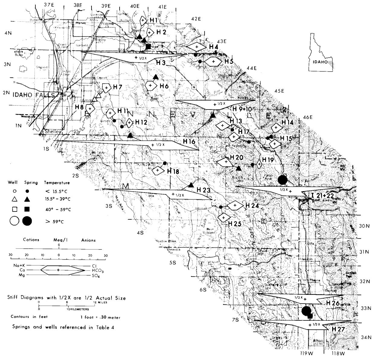
Figure III-5. Stiff diagrams of water chemistries of selected springs and wells in the vicinity of the Caribou Range, southeastern Idaho and western Wyoming
