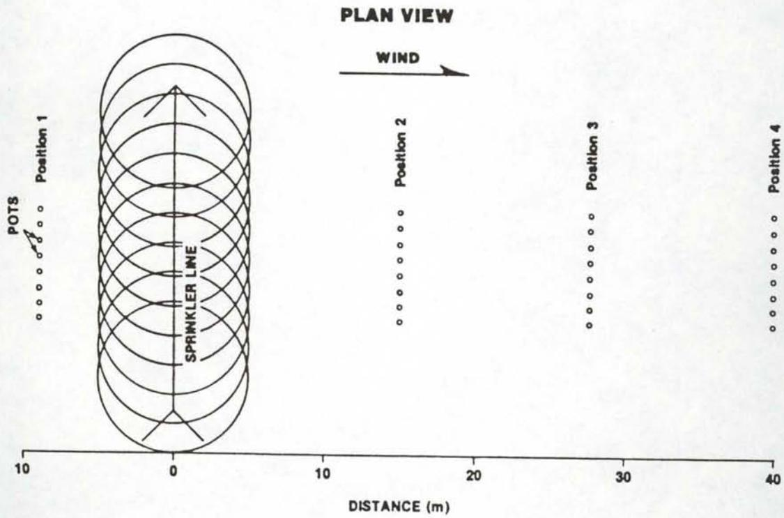
Figure 17. Schematic drawing showing relative locations of sprinkler lateral, pot row positions, and wind direction.
