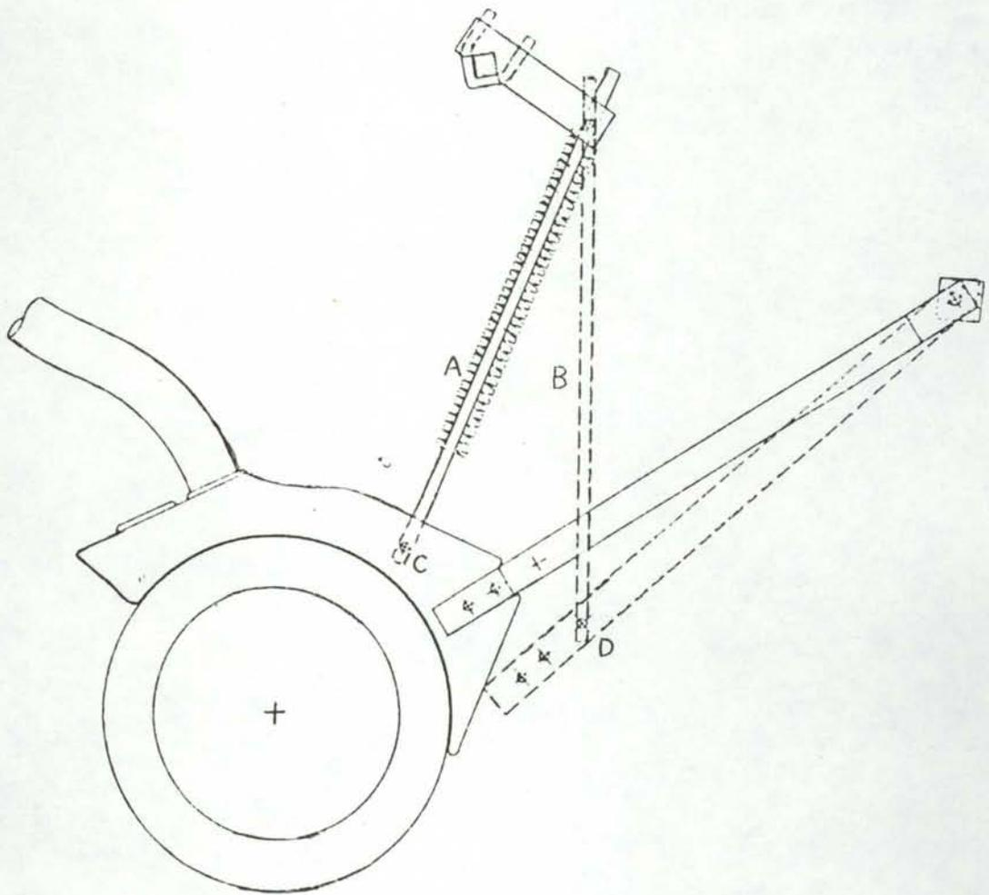
Figure 6. Double disc and hanger. Dotted lines indicate modified position of hanger as drill travels through basins. Note repositioning of hanger attachment point and lengthening of spring hanger rod.
