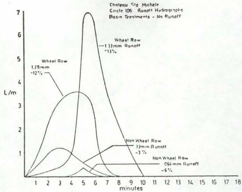
Figure 11. Runoff Hydrograph for check tillage treatment in circle 106
