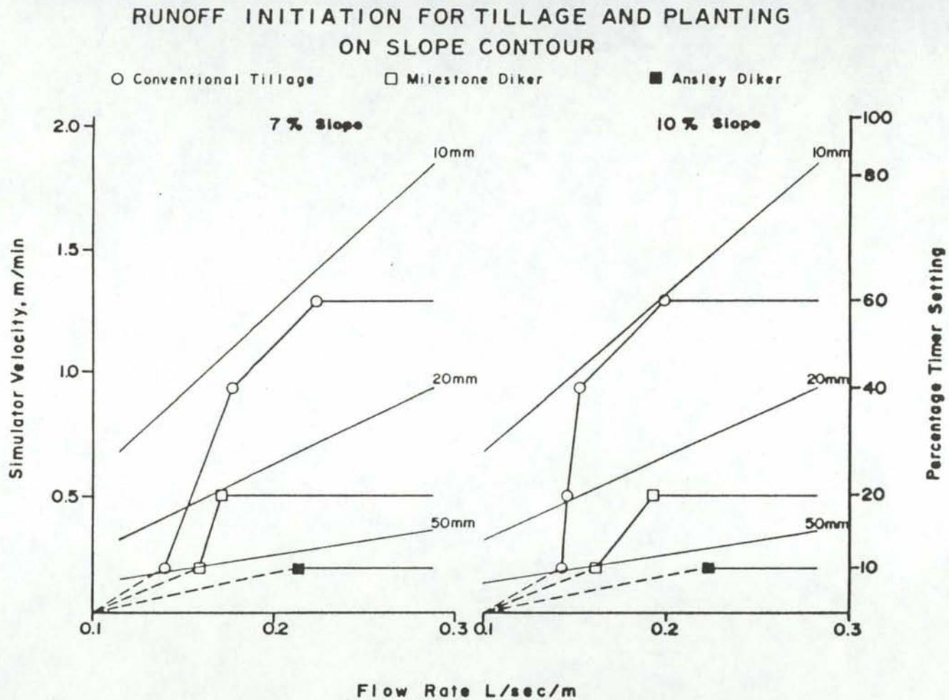
Fig. 8. Results of runoff tests for grain planted up and down slope.
