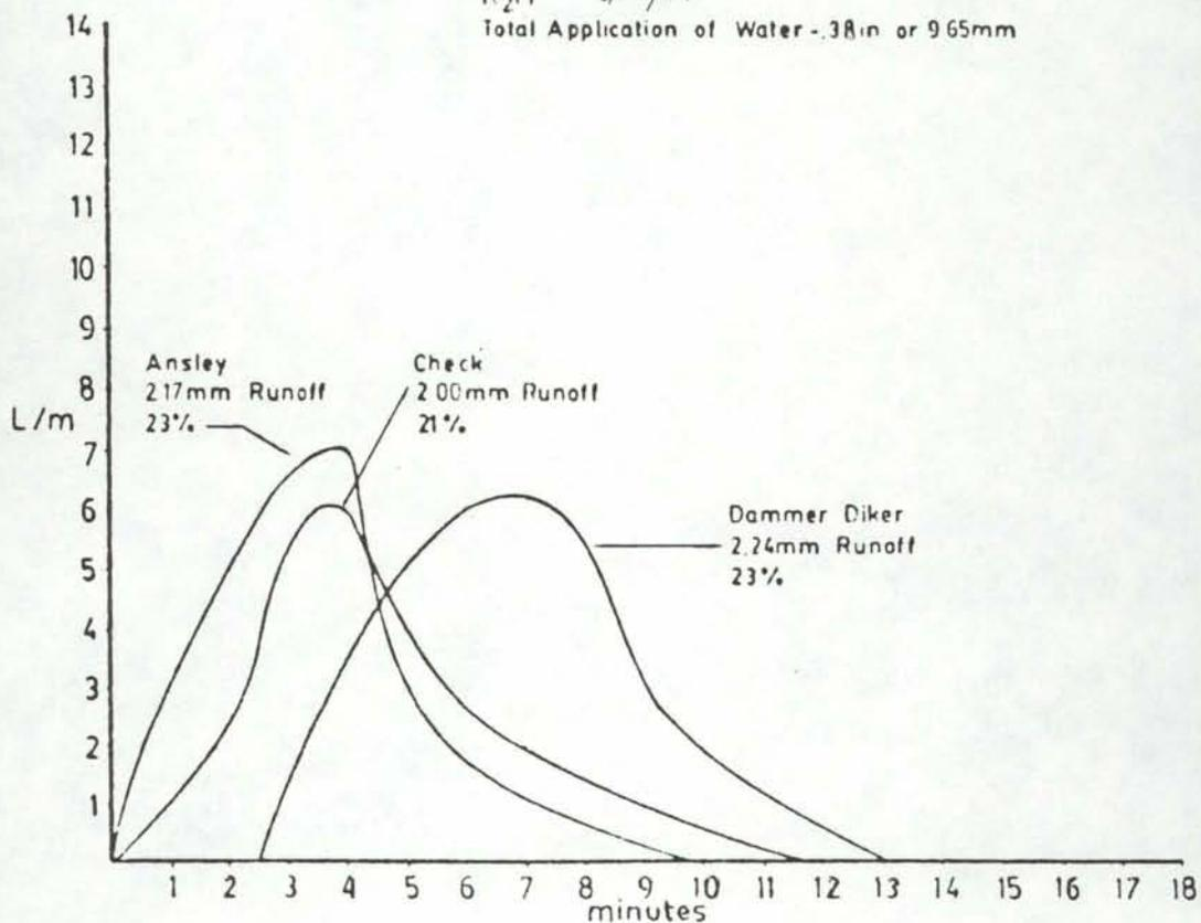
Figure 16. Runoff hydrographs showing little difference in runoff for various potato tillage treatments in late season.
