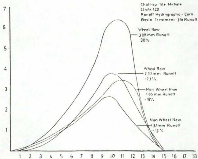
Figure 12. Runoff Hydrograph for check tillage treatment in circle 420
