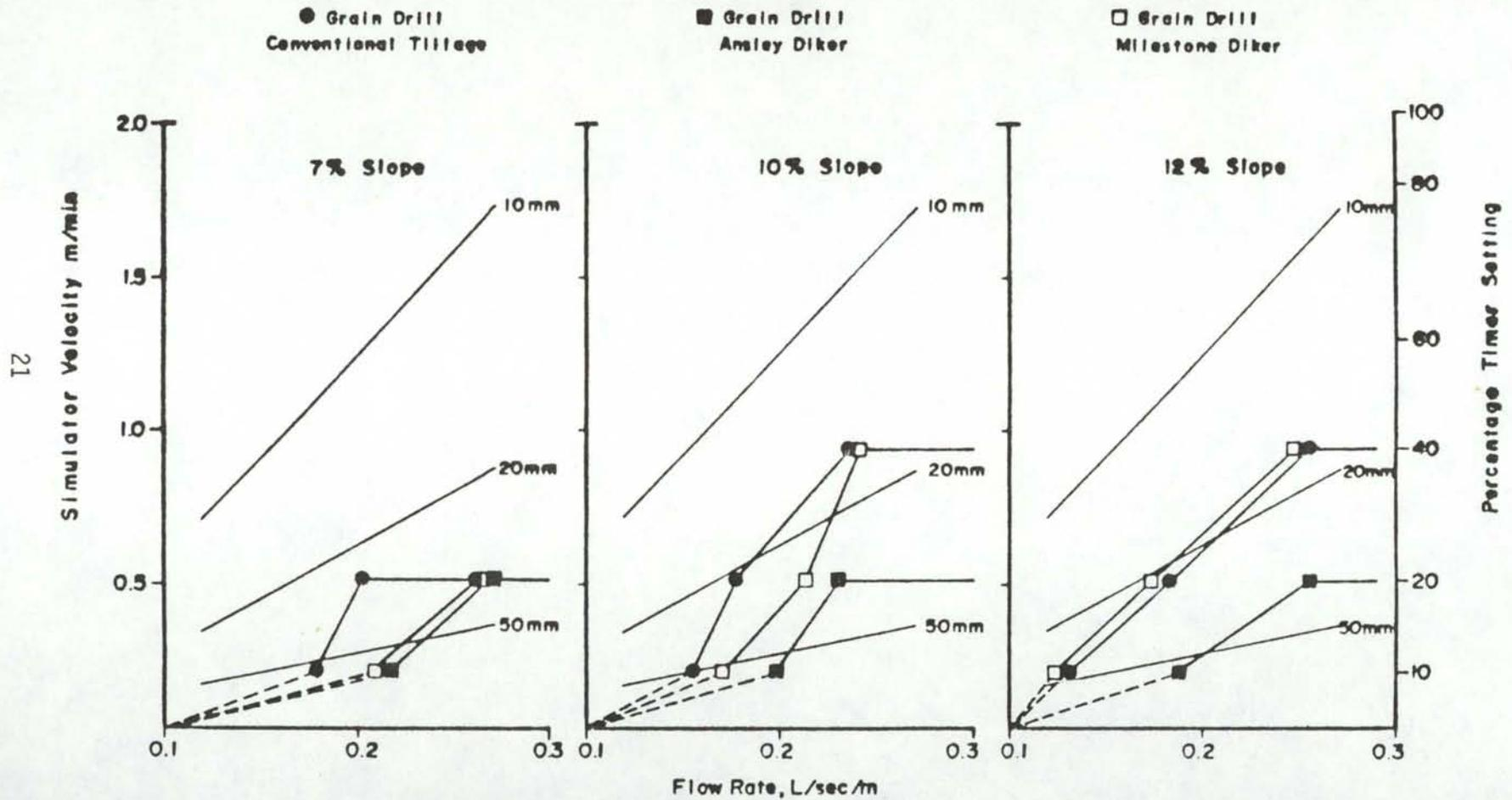
Fig. 7. Results of runoff tests for grain planted on slope contour.
