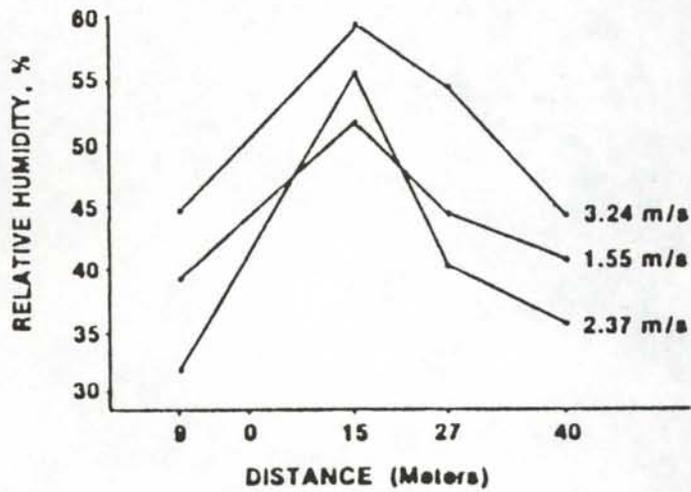
Figure 19. The relationship of RH to sprinkler lateral location.
