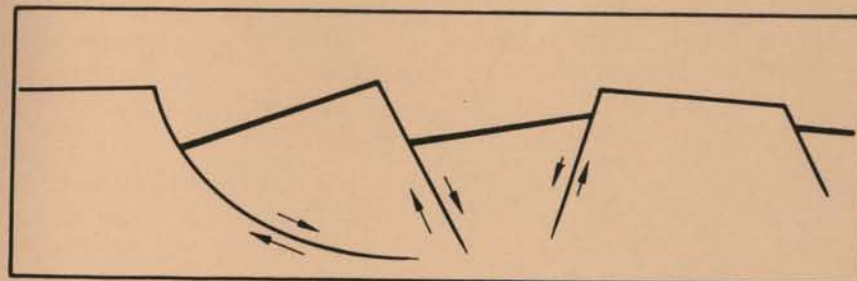
Figure 17. Possible subsurface geometries of basin-range faults.
