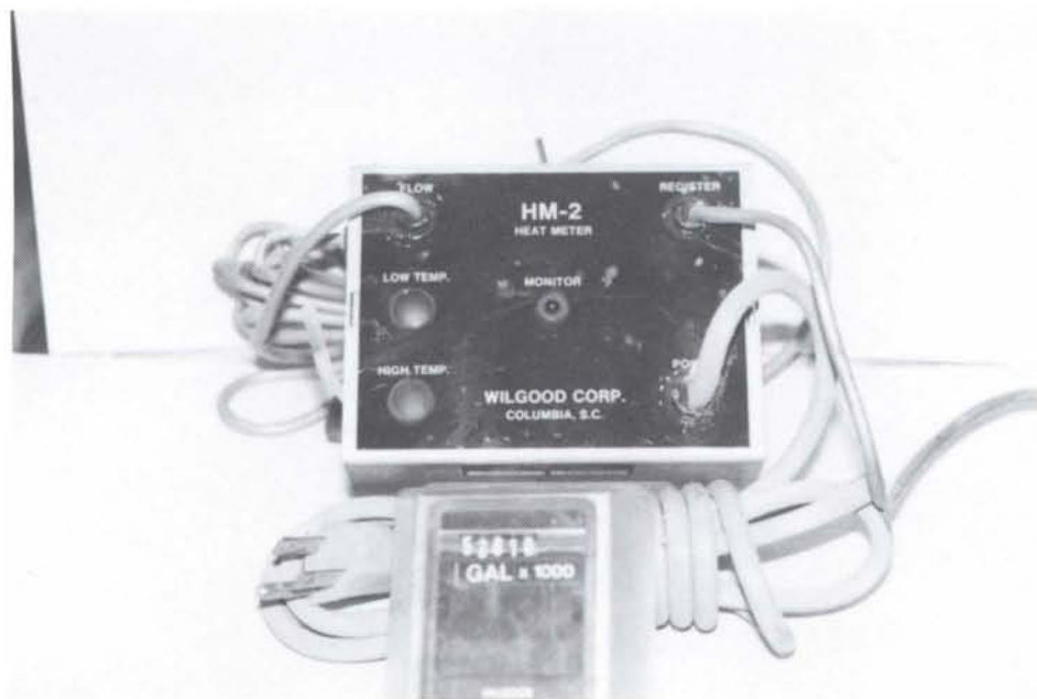
Figure 10b. Wilgood Corporation Dual Turbine Meter Integrator
