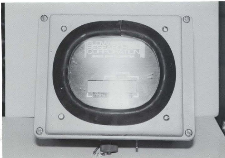
Figure 4b. Flow Research Corporation Flow Meter Integrator
