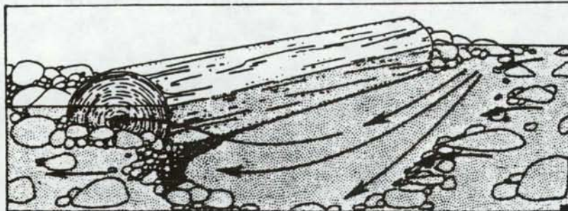
Lateral scour pool associated with large debris.
