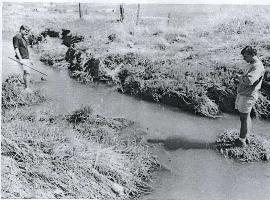
Measuring stream velocity by the float method
