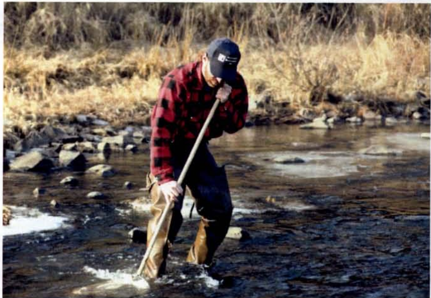
Collection of macroinvertebrate from riffle area using dip net
