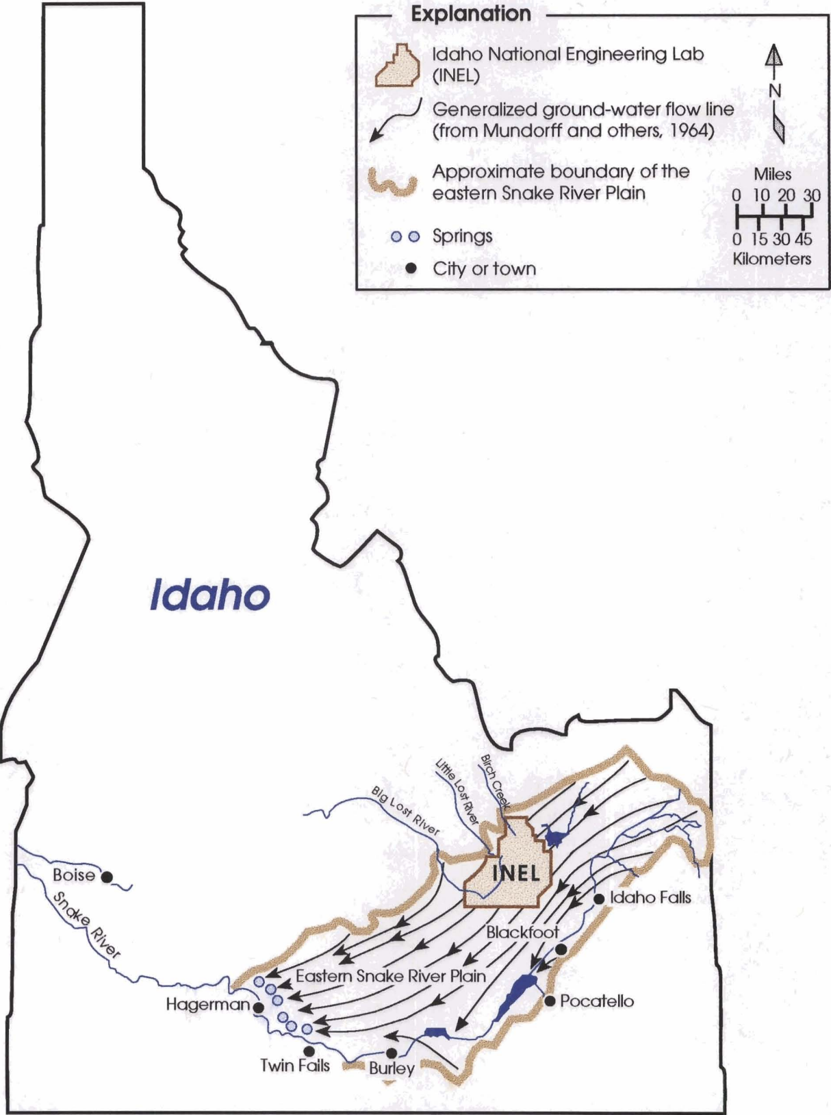
Figure 1. Map of Idaho showing the locations of the INEL, eastern Snake River Plain, and generalized ground-water flow lines of the Snake River Plain aquifer.
