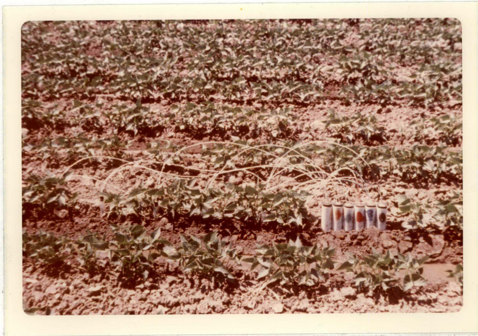
Figure 13 : Soil solution samplers. These samplers allowed samples of the soil solution to be taken at one foot increments, from one to five feet.
