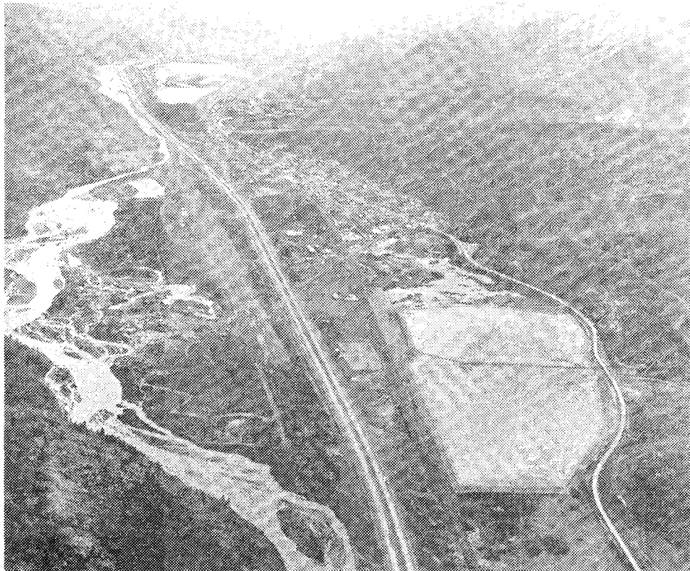
Figure 1. The Valley of the South Fork of the Coeur d'Alene River (March, 1972). Extensive settling ponds now reduce transport of silts to the river. River flow is toward the viewer.
