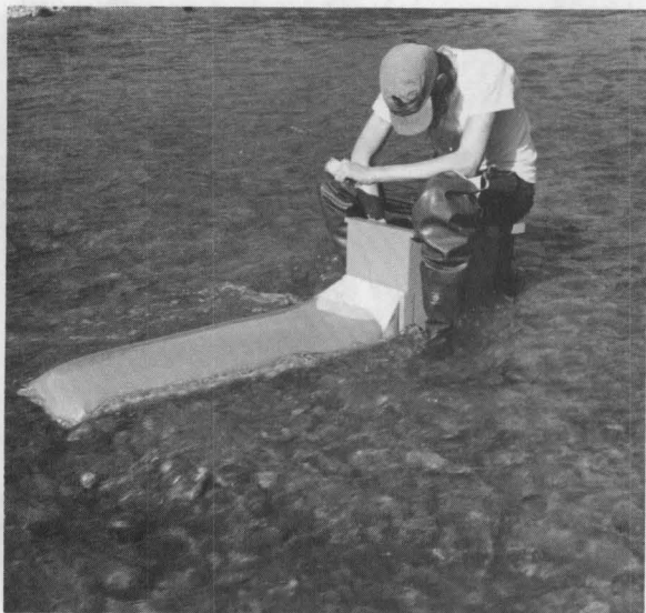
Figure 20. University of Idaho Investigator Operating Mundie Sampler.
