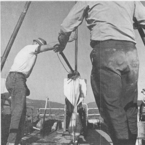
Figure 16. Activation of Trigger Mechanism of Corer.
