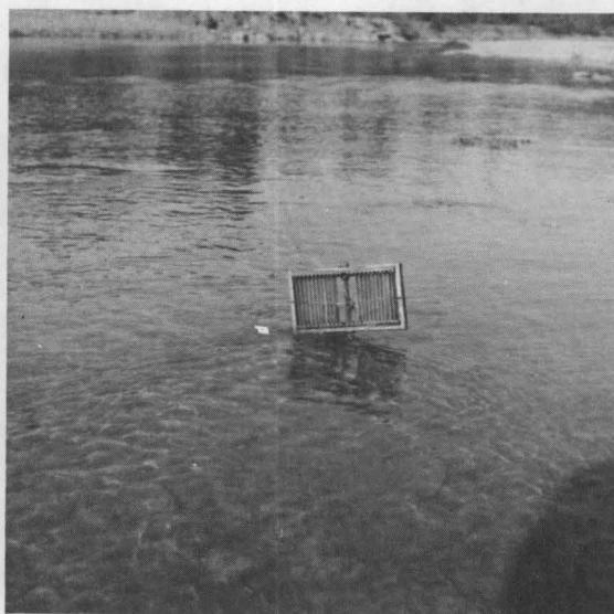
Figure 21. Slide Holder Developed by University of Idaho Researchers for use in Coeur d'Alene River.
