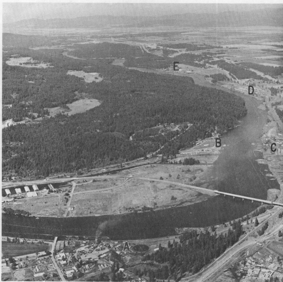
Figure 8. Coeur d'Alene Lake Outlet and the Head of the Spokane River. Letter A Indicates Coeur d'Alene City Sewage Plant, B Indicates the Spokane Yacht Club, and C, D, and E are Industries Along the Spokane River. Flow of River is Away from the Viewer.
