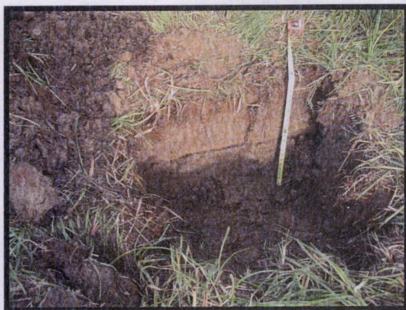
Figure 7. Soil profile near point C along the Black Rock Slough sampling transect. Mottling exists from the soil surface to approximately 10 cm. Note the lack of distinct boundary between the red and gray soils.
