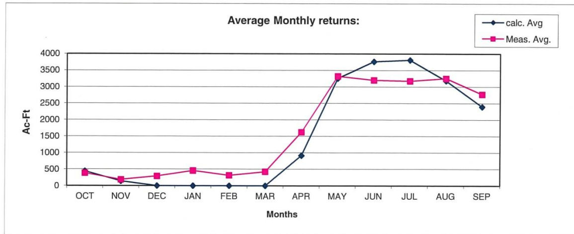
Figure 13. Example calculation of return flow lag factors for Snake River Planning Model.
